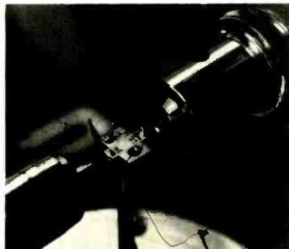
BELL LABS integrated optical device is Fabry-Perot resonator formed by dielectric mirrors on the ends of the electro-optic lithium-niobate substrate material.
