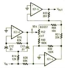
FIG. 2—SIMPLIFIED CIRCUIT of one channel. Cut or boost depends on setting of R52.
