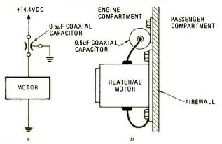
FIG. 6—DC MOTOR NOISE is reduced by adding 0.5- $\mu$ F coaxial capacitor across motor winding as shown in  $\Delta$  Possible mounting location is shown in  $\Delta$
