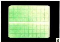
FIG. 1—TIMEBASE KNOB MAY BE LAbeled Time/Cm or Time/Div. At sweep settings longer than 1 ms, the trace (here auto-triggered) flickers or becomes a mere scanning spot.
