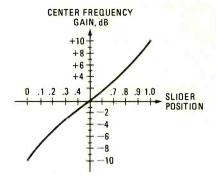
FIG. 4—HOW RESPONSE VARIES with the position of slider on a linear-taper potentiometer.
