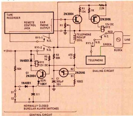
FIG. 1—THE AUTODIALER consists of an ordinary cassette recorder and a few simple components. Pulses recorded on tape dial a selected phone and then a pre-recorded message is played.
