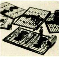
BLOB-BOARDS with prototype circuits built on
