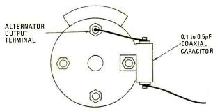
FIG. 4—ALTERNATOR WHINE is reduced by adding 0.1 to 0.5-µF coaxial capacitor to alternator as shown. Check with auto manufacturer for correct value or damage may result. To further reduce noise, an L-section filter can also be added at the input power line feeding the radio.
