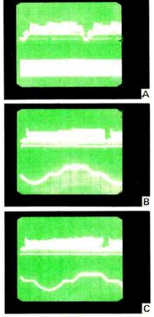
FIG: 3-DUAL-TRACE DISPLAY LOCKS on one signal or the other, unless both are in phases. (a) Horizontal line on trace A, supply ripple on trace B and triggering from trace A; also, timebase is too fast for ripple. (b) Timebase set to accommodate 16.7-ms duration of both TV field and ripple waveform; but slight phase variance lets one crawl. (c) Composite triggering locks both displays despite minor phase difference.
