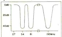
Fig. 3 Harmonic Traps for CB Transceiver
