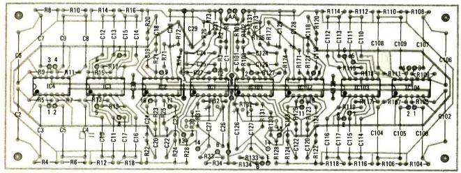
FIG. 7—HOW PARTS ARE POSITIONED on the amplifier board. Right and left halves of board are almost mirror images.
