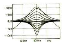
FIG. 3—FREQUENCY RESPONSE of Band 6 as control pot is varied through 11 positions.
