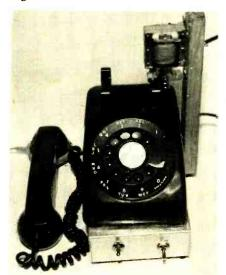
FIG. 2—AUTODIALER WITH SOLENOID that pulses the cradle button. The two toggle switches in the base are not used.
