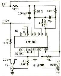
FIG. 3--MONOCHROME MODULATOR for character generator display.
