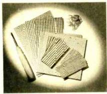
A SELECTION OF VEROBOARDS with various hole sizes, a spot face cutter used to break foil strips and discrete terminals.
