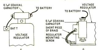
FIG. 5—REGULATOR CAUSED NOISE is reduced by adding a 0.1- $\mu$ F coaxial capacitor in series with the battery terminal. Two possible methods for mounting the capacitor is shown in s and b.
