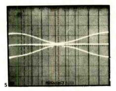
response curve in Fig. 5 was achieved with the tone controls defeated, and in a separate point-by-point sweep, was found to extend from 8 Hz to 40 kHz for the -1-dB rolloff points.
