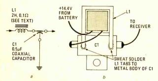
FIG. 9—L-SECTION FILTER shown in a is added to power supply line feeding radio. L-section filter is constructed as shown in b.
