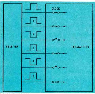
FIG. 2-BIT-PARALLEL TRANSMISSION. All data bits are transmitted simultaneously over five individual circuits.
