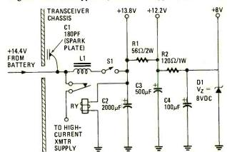
FIG. 7—TYPICAL POWER-INPUT CIRCUIT to mobile radio. If capacitors C1-C4 open up or if L1 should short, noise will enter the radio through the power supply line.
