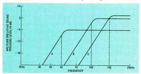
FIG. 1—FREQUENCY RESPONSE can be tailored to different needs. Speaker system A has the best bass response but provides a lower overall output. Speaker system C has a much higher overall output but at a sacrifice in bass response.
