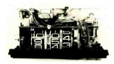
SANKYO 803AL. The digits are printed on translucent drums, driven by a clock motor. A single incandescent bulb lights the number drums from inside. The "chimes" are played by motor-driven music box.
