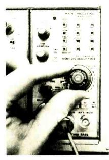
You simply delay the trigger until the signal fed into the oscilloscope reaches line 19 (or the preceding line). To view the VITS signal on lines 17 and 18, you delay the trigger slightly less.
