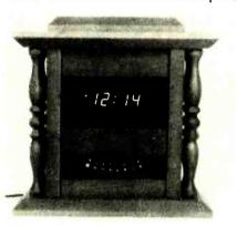
SOLID-STATE TIME. Completed elegant maple mantel-style digital clock with swinging electronic pendulum. Time exposure shows all pendulum LED's lighted.
