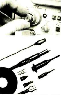
FIG. 2—INPUT ATTENUATOR KNOB calibrates vertical amplifier(s) to measure amplitude of input signal. Low-cap test probe introduces × 10 multiplier that must be taken into consideration.
