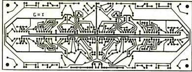
FIG. 5—PATTERN FOR AMPLIFIER BOARD is half-size. Enlarge to exactly 8 inches across.
