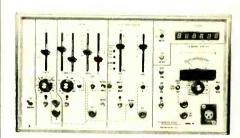
MODEL 101 AUDIO TEST SYSTEM consists of two sine/ square/triangle function generators, pulse generator, frequency counter and AC voltmeter. As a system it will generate a frequency response plot on an X-Y recorder or scope.
