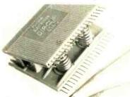
for attaching test probes permits handfree testing. Has nontarnishable nickel-silver contacts; lower contacts measure 1.022 mm wide and mate with DIP contacts, square, serrated upper-end test points measure 0.63 mm and are designed for mini test clips. Nylon casing can withstand temperatures to 240°C. Price: \$19.95.—ITT Pomona Electronics, 1500 E. Ninth St., Pomona, CA 91766.
