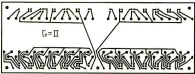
FIG. 6—HALF-SIZE pattern for control board that holds the slide pots.
