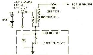
FIG. 3—KETTERING IGNITION SYSTEM was the most common before the electronic ignition system was introduced. Noise suppression involves addding a 0.1- $\mu$ F capacitor on the primary side of the ignition coil and some resistance in series with the spark plugs if the engine does not already have this resistance present. The series resistance can take the form of resistance-type ignition wires or barrel-type resistors that are inserted in the spark plug wires.
