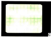
FIG. 1-SIMPLER FEATURES OF SCOPES. such as graticule lighting, often bring more convenience to operation. Shown here are (a) edge lighting, (b) internal graticule, and (c) unique floodgun lighting.
