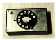
PULSE PROGRAMMER with its electronics (Fig. 3) and telephone dial are built into a small plastic utility box or similar housing.
