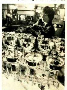
GLASS SURFACES OF PHOTOMULTIPLIER TUBES being treated at RCA Electro-Optics and Devices plant in Lancaster, PA. When installed in nuclear detection instruments, tubes can "see" nuclear radiation as blue flashes of light.
