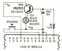
FIG. 7—ALARM DRIVER and seconds display switch added to Solid-State Time's clock.
