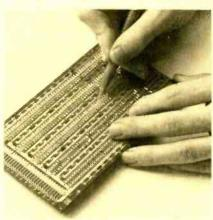
A VEROWIRE PEN being used to route heat strippable wire on a DIP board.
