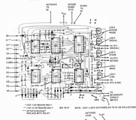
FIG. 8-COMPONENT PLACEMENT diagram.
