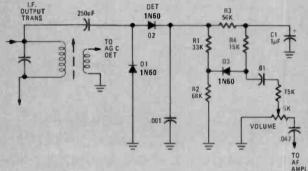
FIG. 4—SERIES-GATE ANL circuit used on the Pace model 133 transceiver.
