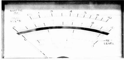
FIG. 2-AUDIO METER has dB scale referenced to 1 voit.
