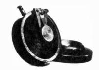
THE FIRST CONTACT MICROPHONE. The upper photo is the original microphone of 1877; the lower one is the form in which it was used as a telephone transmitter. Emile Berliner's microphone used a metal-to-metal-contact; Edison's used carbon contacts.
