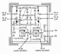
FIG. 3—COMPONENT PLACEMENT diagram.
