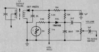
FIG. 5—SERIES-GATE ANL circuit. This version is used on the Johnson Messenger model 123A.
