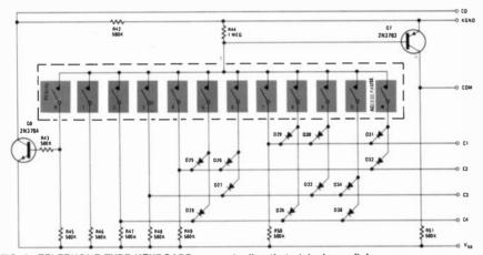
FIG. 2—TELEPHONE-TYPE KEYBOARD connects directly to telephone dialer.
