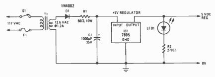
FIG. 3—REGULATED POWER SUPPLY is suitable for TTL and CMOS IC's.
