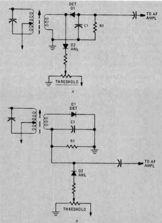
FIG. 3—TWO SHUNT-TYPE PEAK NOISE LIMITERS. These are not as effective on ignition noise as the series type.
