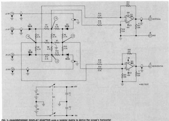
FIG. 1—QUADRIPHONIC DISPLAY ADAPTER uses a resistor matrix to derive the scope's horizontal and vertical signals.
