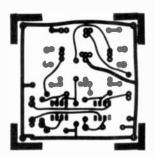
FIG. 2-FOIL PATTERN is shown half-size.
