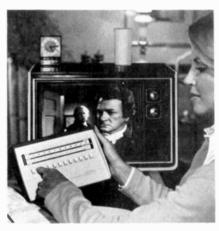
without motors, this solid-state unit provides direct-access channel changes, fine tuning and remote on-off of a TV set from anywhere in the room. The device consists of two units; an all-channel converter and a control unit interconnected by a 25-foot, plug-in, control cord. The converter is connected behind and beneath
