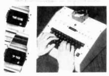
Modules for this type of watch, with a five-word message pre-programmed during manufacture, were first announced by Hughes early in 1976. The present watch (also a Hughes module) differs in that the user can set up and change his own message at will without having to send it back to the factory.
