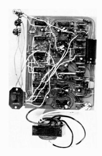
HII INFINITION IS A MUSIC GENERATOR THAT uses pink-noise sources to select the pitch and duration of each musical note. The pitches are selected from three octaves of a pentatonic scale. Most Eastern music is based on the pentatonic scale which has five notes per octave with simple frequency ratios. Eastern music lacks much of the formal structure of Western music and is most successfully imitated by simple pink-noise sources.
