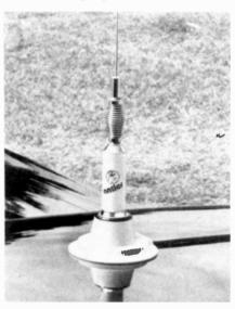
antenna mounted on the center area of the roof of a truck cab is 3 dB above isotropic. The average VSWR is less than 1.3 without making any attempt to optimize this figure. Model A-280 is base-loaded, mobile, magnetic-mount with a 47-inch heat-treated, stainless steel whip. Antennas are factory matched to resonate at 146 MHz. A chart is provided allowing adjustments ranging from 144 MHz to 156 MHz.—Antler Antennas, 6200 South Freeway, Fort Worth, TX 76134
