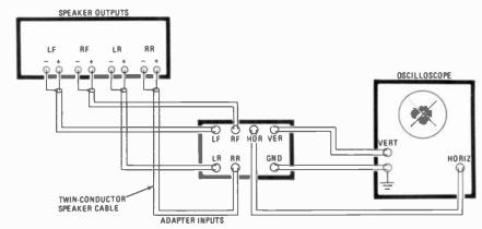
FIG. 4-HOOK-UP of the scope adapter.
