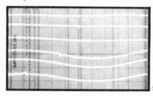
loudness compensation applies only to the bass end, while the moderate amount of treble boost incorporated in the loudness circuitry remains constant regardless of the CONTOUR control position.
