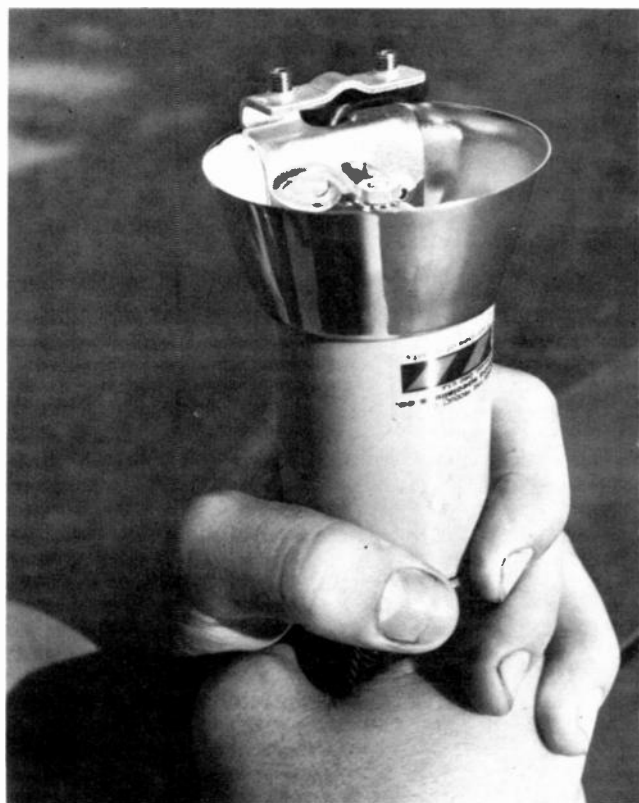
FIG. 1—INDENTED CHANNEL prevents damage to the transmission line when the trunk is closed.
