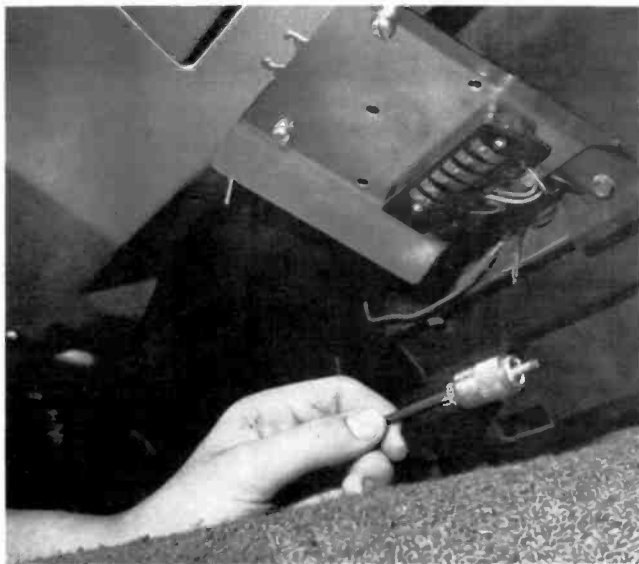
FIG. 7—TRANSMISSION LINE should be just long enough to reach the transceiver. Excess should be left in trunk, not under the dash where it can get tangled with the driver's foot.
