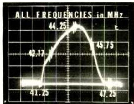
FIG 4—NORMAL IF response of color receiver.
