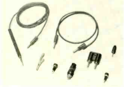
FIG. 9—SOME OF THE low-frequency test cables and connectors in common usage today.
