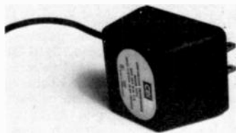
FIG. 4—PHOTO OF THE PLUG-IN TRANSFORMER Model LVT-1. This UL listed device steps the line voltage down to a safe 12-volts ac and is used to power all three clocks described in this article.
