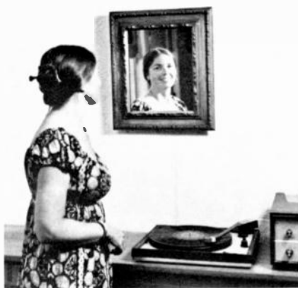
MIRROR LOUDSPEAKER. The flat speaker concealed within the mirror frame causes the suspended mirror to vibrate and act as a secondary sound source.
