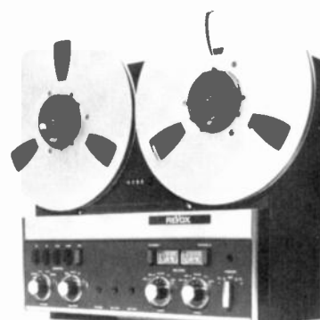
FIG. 8—THE REVOX REEL-TO-REEL tape recorder has capability of handling 10-1/2 inch reels and comes with a torque-changing switch to allow smooth handling of either these larger reels or the smaller 7-inch types.
