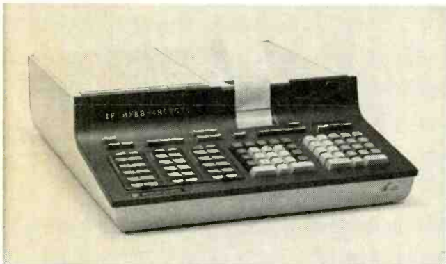
A FULLY PROGRAMMABLE ELECTRONIC CALCULATING SYSTEM, the Hewlett-Packard 9820A, with a built-in printer. This versatile machine represents the pinnacle in electronic desk calculators and offers many of the capabilities of a true minicomputer. The three keyboards to the right of the central arithmetic portion of the machine can be "user defined" by means of plug-in read-only memory modules.
