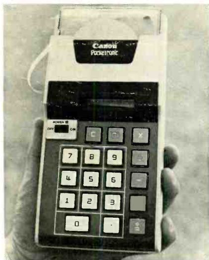
THE CANON POCK-ETRONIX is the only portable electronic calculator with a paper tape printout. This novel machine incorporates Texas Instruments MOS LSI circuitry but is manufactured in Japan. Texas Instruments also manufactures the semiconductor thermal printout device. The paper tape can be replaced almost instantly by plugging in a new cassette.
