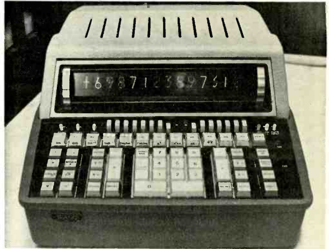
WANG SERIES 100 ELECTRONIC DESK CALCULATOR. Manufactured by the first company into the electronic desk calculator business, the machine includes scientific and statistical keys as well as interfacing for an optional printer. The display panel is on an axle and can be rotated for convenient viewing by the user.
