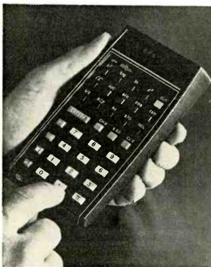
THE MOST ADVANCED POCKET CALCULATOR made today—the Hewlett-Packard HP-35. This sophisticated electronic slide rule has trig functions, a memory, and can take square roots. It also handles logs and exponential terms. The HP-35 represents a major breakthrough in miniature electronic calculating machines.
