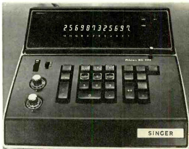
A LATE MODEL DESK CALCULATOR , the Friden EC1117 has memory capability. Low-cost machines like this are popular with businesses. Friden also manufactures printing calculators and all electronic cash registers.
