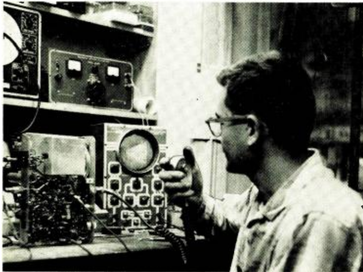
Trapezoid pattern is good speedy modulation check (see Fig. 2). For information on how to interpret it, try Radio Amateur's Handbook or other books on transmitter design and maintenance.
