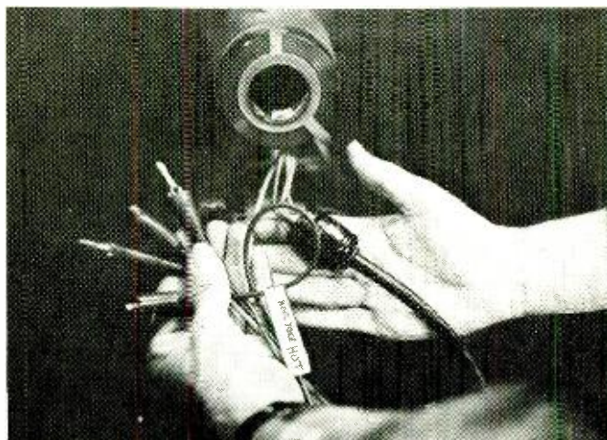
Fig. 5—Make up socket and cables to fit Whatsit's yoke plug. Put clips on the ends of the wires and mark the hot lead of the horizontal deflection coils with a tag.
