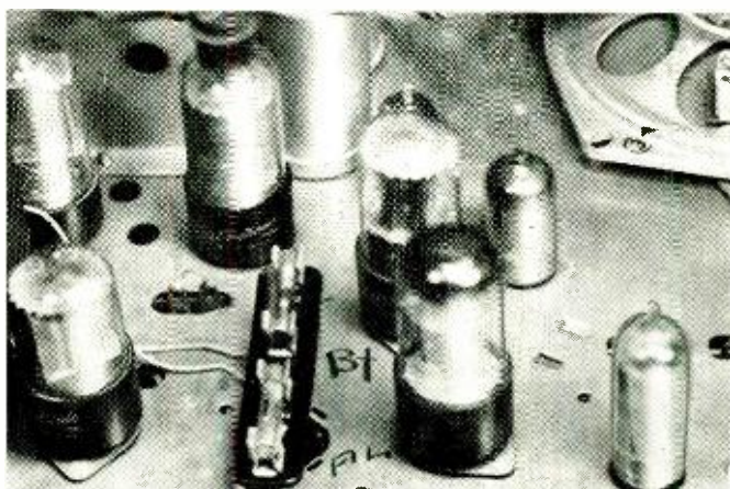
Fig. 6—Put a couple of old fuse holders in the power supply circuits of the Whatsit, one in B-plus and the other in the heater circuit. Use 20-amp fuses—they aren't for protection, just simple quick disconnects. Clip to the ends of the fuse holders to pick off power.
