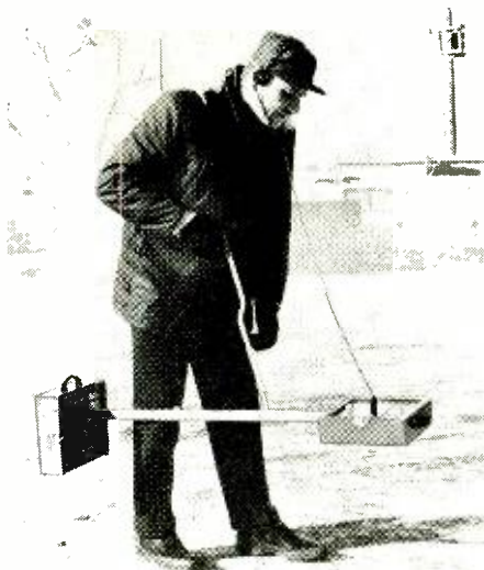
Coupled together, rf transmitter and receiver can be used by one man for finding large, deeply buried objects.
