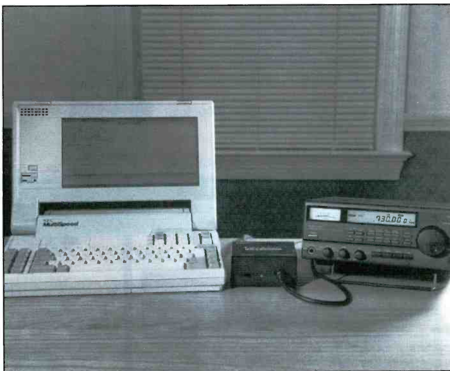
Figure 1. The "budget" spectrum analyzer: laptop computer (left), interface unit (middle), and general coverage digital radio (right).
