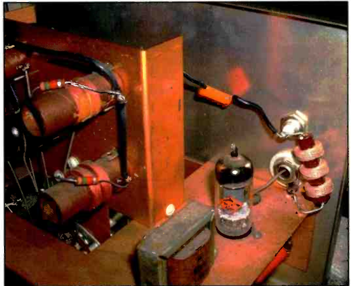
Photo G. Adding a 200- \mu H to 2.5- \mu H RF choke between ground and the frequency counter BNC fitting effectively removes any residual audio signals from the RF output.
