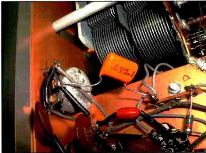
Photo F. The problem shown in Photo D can be partially alleviated by making the AM modulation level settable by the operator. Rerouting the audio path to do so simply involves moving the connections for a .01 capacitor under the SG-8 chassis.
