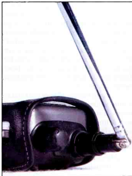
A handy angle connector like this one allows the radio to sit flat on a console and still get the antenna above the dashboard. Some Velcro can help hold it in place if necessary.
