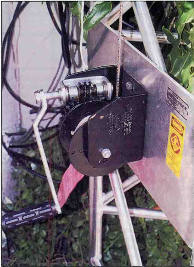
The worm gear crank assembly is easy to turn, but very slow in raising and lowering the tower.
