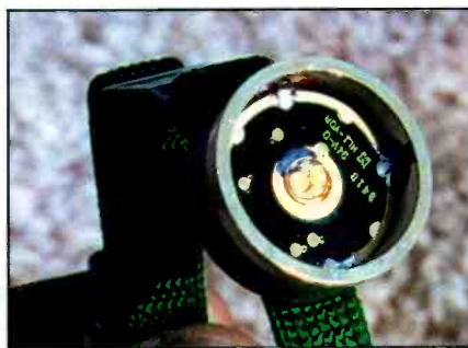
The 218-MHz radio tag with battery removed.
