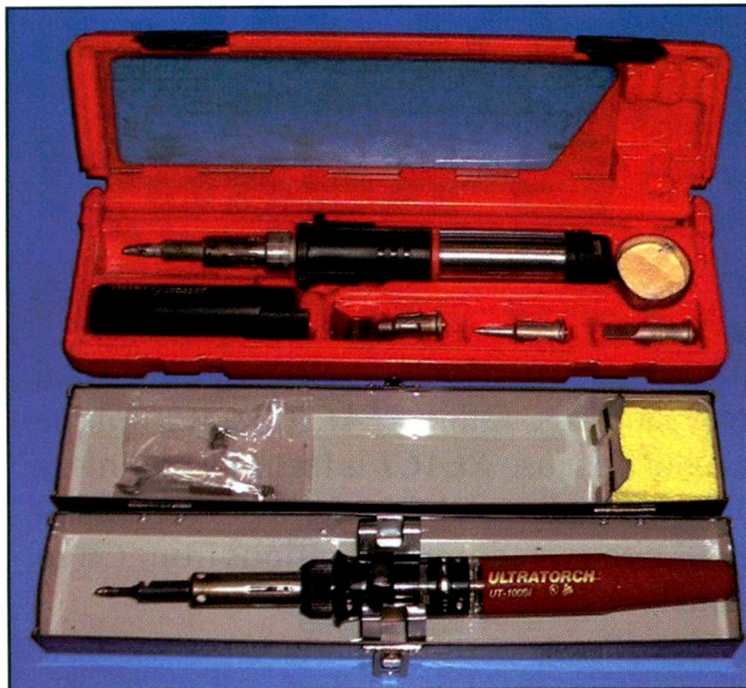
Photo A. The Weller Portasol PSI-100K portable butane soldering tool kit (upper unit) and the Master Appliance Ultratorch UT-100Si soldering tool kit (lower unit) are my personal units and have undergone two or three years of field testing. Both do the job.
