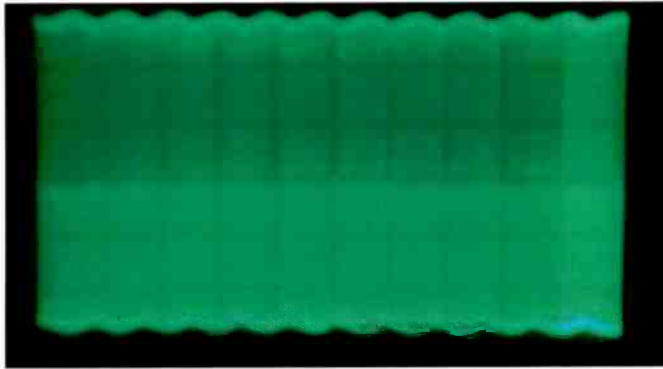
Photo E. The maximum AM modulation percentage was at best a few percent on the lower three ranges (A, B, and C) on the author's SG-8.
