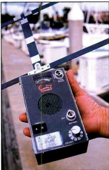
The Com Spec receiver with optional Moxon directional antenna.
