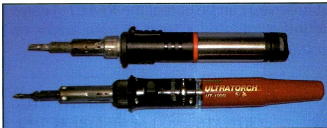
Photo B. Here’s a better view of both irons (Weller, top; Master Appliance, lower) out of their carrying kit cases. Both irons feature piezo ignition, variable heat settings, and fuel level viewing windows.
