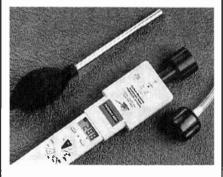
The head slides onto the DMM to convert carbon-monoxide concentration in parts per million (ppm) to mV (millivolts) DC. Setting the meter on 200-mVDC or 2000-mVDC range displays carbon monoxide in ppm, with an accuracy of 5% ±3 ppm. The easy-touse head is small and lightweight and has a long battery life. The catalytic sensor has been known to last for more than seven years and remain properly calibrated; life and accuracy may vary depending upon use, abuse, and exposure to harmful chemicals.
