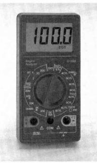
The 3-1/2 digit, 2000-count multimeter measures voltage, resistance, amps, rpm, duty cycle, and dwell, and performs diode tests. Its large LCD readout features a unique sub-display continued on page 74
