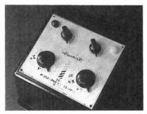
This 1906 Lionel transformer eliminated the need for batteries and permitted the speed of toy trains to be easily adjusted.
