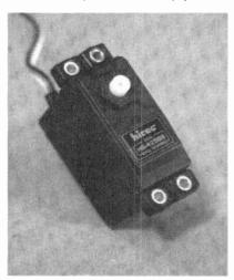
Fig. 3. Here's one of the Hitec HS-425BB servos used in the author's prototype.
