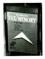
The FMM card features a battery-saving, ultra-low-power sleep mode; built-in interface software; flash memory to upgrade the modem's operating program code on-line; and builtin DAA line-interface circuits.
