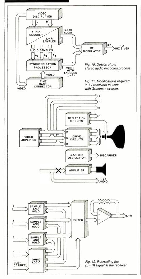
ing the familiar algebraic addition and subtraction, (L + R) + (L - R) = 2L and (L + R) - (L - R) = 2R. In actual practice, some time delay must be added in the (L + R) channel to equal the processing delay of the (L - R) channel.
