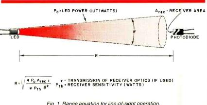
Fig. 1. Range equation for line-of-sight operation.
