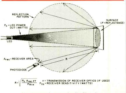
Fig. 2. Range equation for operation with a diffuse reflector.
