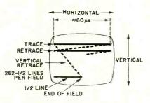
Fig. 3. How the image is formed on a CRT screen by scanned lines.
