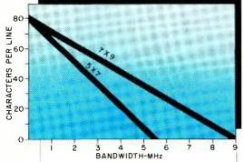
Fig. 4. How bandwidth and characters per line are related.
