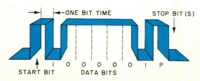
Fig. 3. Diagram of a typical serial data transmission.
