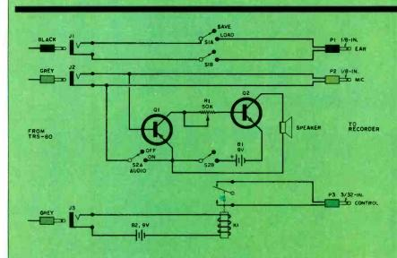
The three circuits operate independently between cassette and computer.
