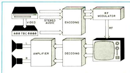
Fig. 9. Block diagram of closed-circuit stereo audio demonstration by Grumman.
