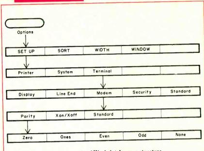
Fig. 1. A sample of Workslate's menu structure.
