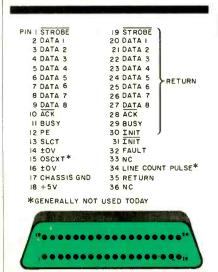
Fig. 1. Pinout of a Centronics parallel connector.
