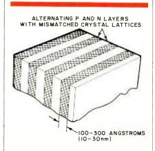
Fig. 8. Formation of a simple strained-layer superlattice device.
