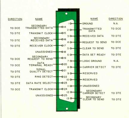
Fig. 4. Pinout of an RS-232 serial connector.
