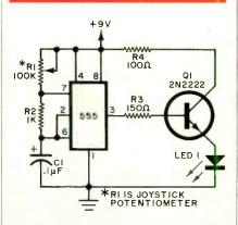
Fig. 5. Single-channel near-infrared joystick transmitter.
