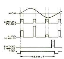
Fig. 7. Audio is sampled three times per horizontal line (bottom) and encoded into a single 2-µs signal.
