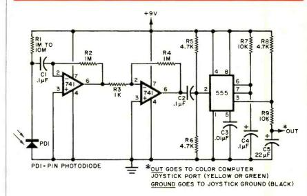
Fig. 6. Single-channel infrared-coupled joystick receiver.
