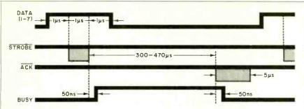
Fig. 2. Timing chart for a Centronics parallel interface.
