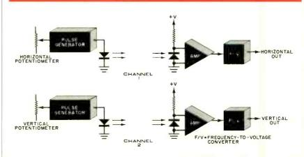
Fig. 4. Block diagram of infrared computer-joystick interface.
