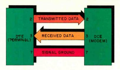
Fig. 5. The basic RS-232 connection uses only three lines.
