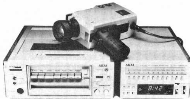
Typical portable setup has recorder, tuner-timer and color camera, as in this Akai Activideo system.
