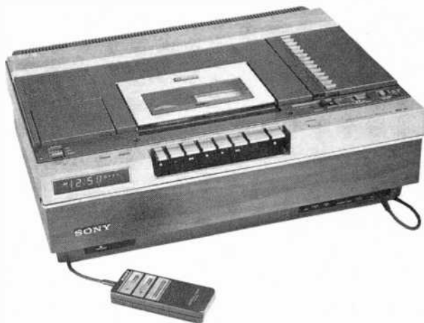
Sony SL-5600 has visual fast-search and can record up to four different programs over a 14-day period.
