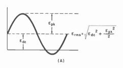
Fig. 4. Rms value of sine wave can be calculated as described in text using diagrams shown here.
