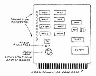
Fig. B. Layout of the major components of the experimental oscilloscope on a 2 x 22 connector edge board.
