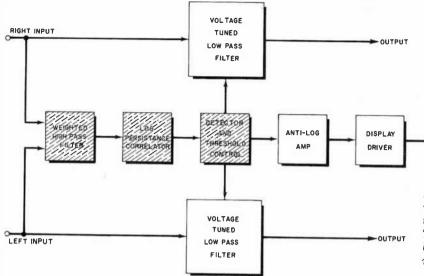
Fig.1. Block diagram shows how input signals are processed to generate a control signal. This signal governs filter's break frequencies to pass music but attenuate noise.
