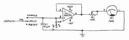
Fig. 1. Schematic of a demonstration sample/hold circuit.
