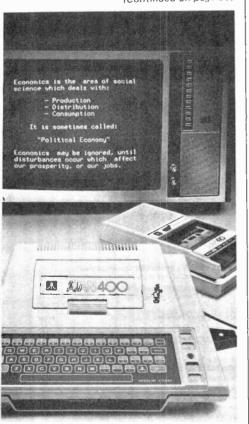
The Atari-400 personal computer uses a 6502 CPU, 8K of RM and 8K of ROM. Keyboard is a 56-key Monopanel with touch-control points. RCA 1802 COSMAC CPU
