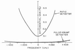
Fig. 3. Differential gain vs. frequency for ratio detector and pulse-count detector showing distortion performance.
