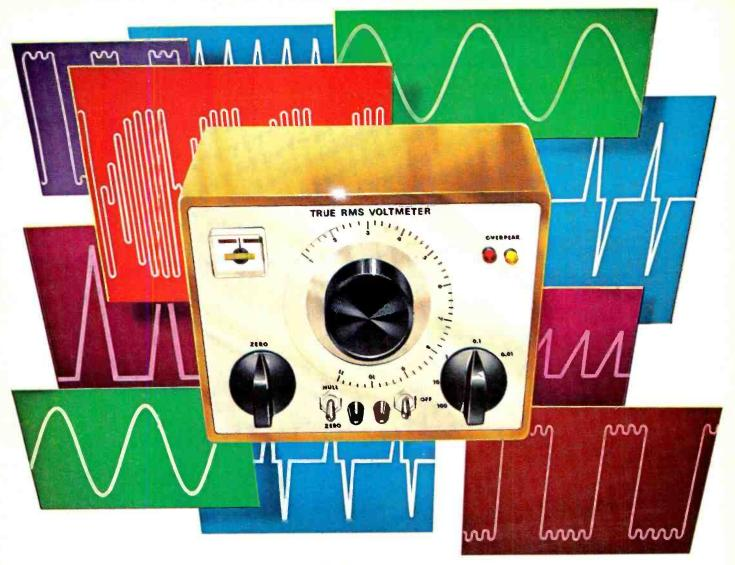
VENTUALLY, most serious electronics experimenters find a need to measure the power content of an odd-shaped waveform. This might occur in measuring the output of a class-C amplifier, audio, video or noise signals; power supply inverter waveforms; or just plain power supply ripple.
