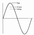
$V_{PK} = 1.414V_{RMS} = 1.569V_{AVG}$   $V_{RMS} = 0.707V_{PK} = 1.110V_{AVG}$   $V_{AVG} = 0.637V_{PK} = 0.901V_{RMS}$ VOMs read 1.110V<sub>AVG</sub> VTVMs read 0.707V<sub>PK</sub>
