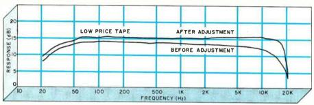
Fig. 3. A low-price tape shows obvious deficiencies in performance, but is much improved in any case after the adjustment sequence.
