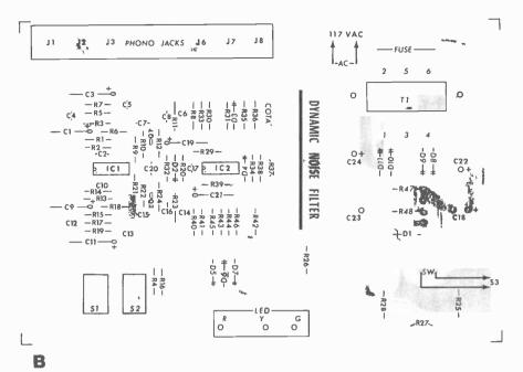
Fig. 4. Actual-size etching and drilling guide for the "Silencer." Board is shown at (A); parts placement at (B).
