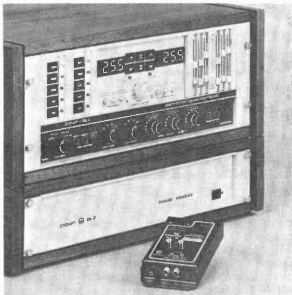
The complete control system, as shown here, includes the control center, power-supply module and separate modules for each phono cartridge input.
