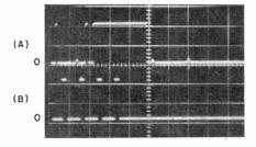
Fig. 7. Scope trace (A) shows switch bounce, while (B) shows four pulses initiated by switch closure. Sweep time is 50 μs/div.
