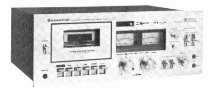
Deck features a vernier bias adjustment, two test oscillators, and bias and equilization switches which allow a precise match to any tape formula.
