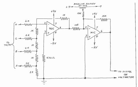
Fig. 4. Schematic of an improved D/A converter.
