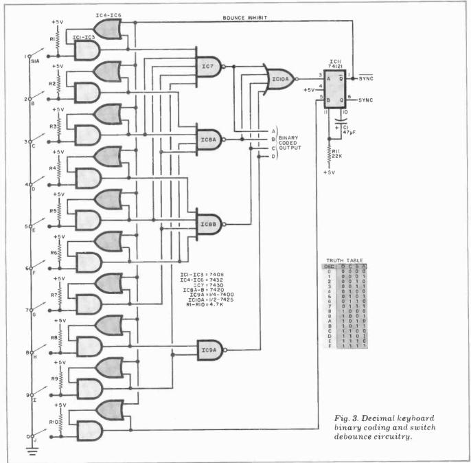
Referring back to Fig. 3, when all keyswitches are open, their associated AND gate (*IC1* through *IC3*) inputs are high. Hence, the outputs of the four encoding NAND gates (*IC7* through *IC9*) are low. Closing any keyswitch except 0 forces at least one of the NAND gate inputs high.
