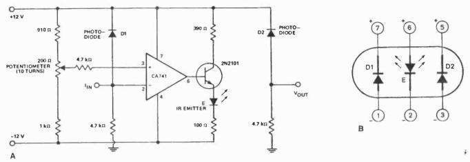
Fig. 4. RCA's C30121 optically coupled isolator: (A) driver circuit; (B) lead connections.
