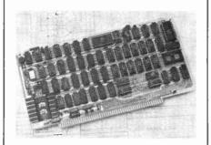
ics. It has its own screen-refresh memory and latched eight-bit parallel port, is S-100 compatible, and video output is available as composite video or separate video and sync. \$195 kit, \$235 assembled.
