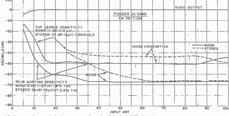
Noise and sensitivity curve for the Model GX-5050.
