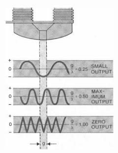
Fig. 2. Tape head output peaks when wavelength  $(\lambda)$  is 2X head gap width (g), drops to 0 when both are equal.
