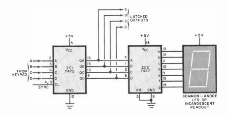
Fig. 11. Latched output for a keypad. Display is on a 7-segment LED readout.
