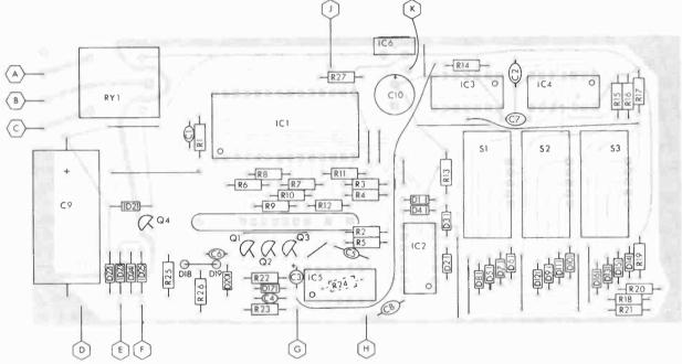
Fig. 2. Full-size etching and drilling (A) and parts placement (B) guides for a suitable printed circuit board.
