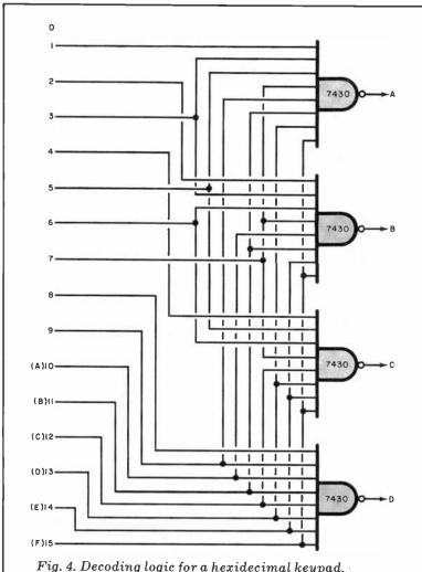
Fig. 4. Decoding logic for a hexidecimal keypad. This circuit is an addition to that in Fig. 3.
