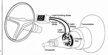
ple, has developed a photo-cybernetic system to monitor vehicle speed, eliminating less reliable mechanical linkages. Readout is by digital LED's. And just imagine what the potential clock rate of a computer would be with no impedance in interconnecting circuitry! Clearly, it's a technology whose time has come.
