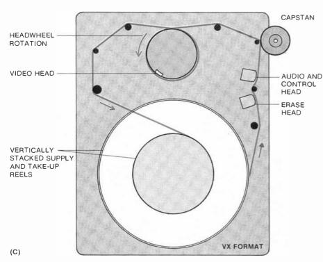
Fig. 7. Various ways of video-tape passage through VCR machine: (A) Betamax's modified "U-load;" (B) simpler "M-load" used by VHS; (C) "Alpha-wrap" on Quasar's VR-1000.
