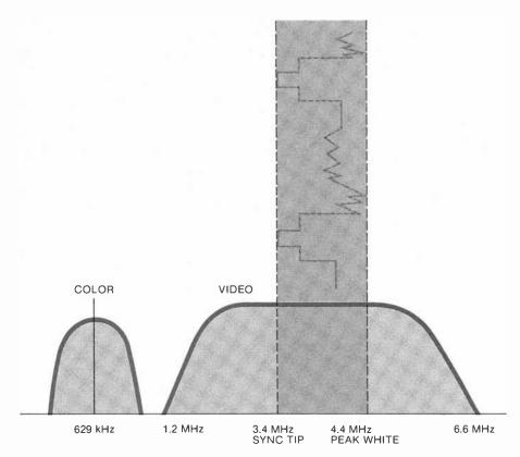
Fig. 1. Video signal spectrum of typical VCR.
