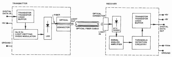
Fig. 1. Block diagram of RCA's C86003E fiber-optic data link.
