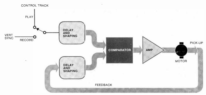
Fig. 6. Vertical sync signal on control track controls playback motor speed so video heads scan correct video tracks.
