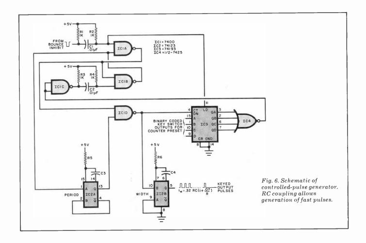
allow rapid action—in fact, a complete pulse train can be generated within the width of the sync pulse. Without RC coupling, the latch would be locked for the duration of the sync time. A transient input is a must to avoid lockout. The *IC3* down counter has its LOAD enable input RC coupled to the sync input. This input requires a transient input to operate.
