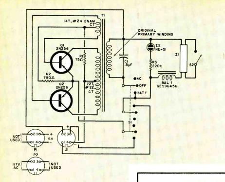
Fig. 1. Two-transistor power oscillator generates approximately 110 volts for ultraviolet lamp.
