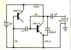
reverse-biased pn junction of a 2N2712 transistor is used as a noise generator. The second 2N2712 is an audio amplifier. The 0.005-µF capacitor across the amplifier output removes some high-frequency components to simulate pink noise more closely. The audio output may be connected to high-impedance earphones or to a driver amplifier for speaker listening
