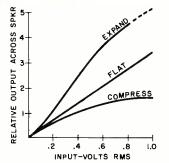
Fig. 2. Graph shows how compander expands or compresses the relative output across speaker.
