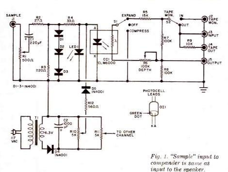
C2-1000-µF, 15-volt, electrolytic capac-D1 to D5-1N4001 diode (or similar)\* J1 toJ5—Phono jack\* LED1—MV50 light emitting diode (or similar)\* OII-Optical isolator (Clairex CLM6000
