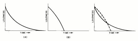
Fig. 1. Curve (A), left, shows reverberation characteristics of a large hall; (B) is for small listening room. Fig. 2, right, combines them to show how time curve (B)'s acoustics dominate recorded ambience.
