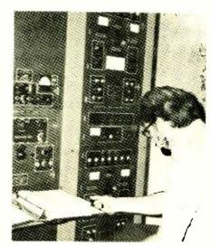
Technician checks that radiation pattern of his VOR system is within tolerances required by the FAA for radio-navigation.
