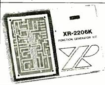
The Function Generator Kit features sine, triangle and square wave; THD 0.5% typ.; AM/FM capability.
