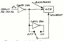
Fig. 3. Practical circuit for driving an LC display.
