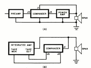
Fig. 3. If you have separate preamp and power amplifier, use hookup at (A). For integrated amplifier, use (B). Both are for one channel only.
