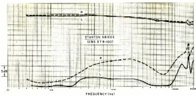
sponse, we temporarily increased the load to 480 pF, which is as high as will ever be encountered in practice. This increased the drop rate in the output curve at frequencies beyond 10,000 Hz, amounting at 20,000 Hz to an additional 5 dB. The Model 681EEE obviously does not require excessive circuit capacitance to equalize its frequency response as do some other cartridges. It should deliver optimum performance with almost any load.
