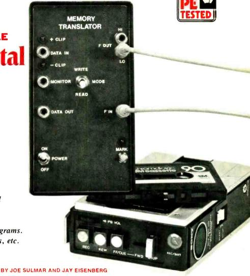
HE portable Memory Translator described here is designed to convert do and low-frequency information to a signal that can be recorded on almost any low-cost cassette. This permits the storage of data (including digital) of a number of different types for future use and reference. (An alternative is the use of a chart recorder—which is not usually portable and is relatively expensive.)
