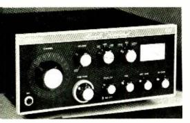
Y-GAIN'S Model 623A base station Citizens Band transceiver is designed for both AM and SSB operation. In some respects, it differs from other AM/SSB rigs. For example, the circuitry is all solid-state in design, except for the transmitter's power amplifier stage, which is a vacuum tube. This design departure greatly reduces the chance of damage to the power amplifier due to mismatched loads.
