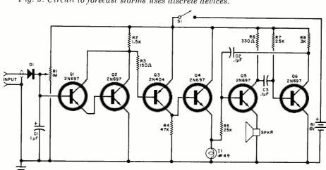
Fig. 5. Circuit to forecast storms uses discrete devices.
