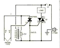
Q1, is not given a specific part number since various loads demand different currents. Check how much current your load demands and obtain a triac that can handle this amount. The triac should be well heat-sinked. Use the same current rating for F1 as Q1, and make it a quick-acting type fuse. The resistors may be mounted on a board, with leads in the clear used as probe tips.
