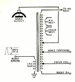
Flyback transformer has special winding to generate spikes.
