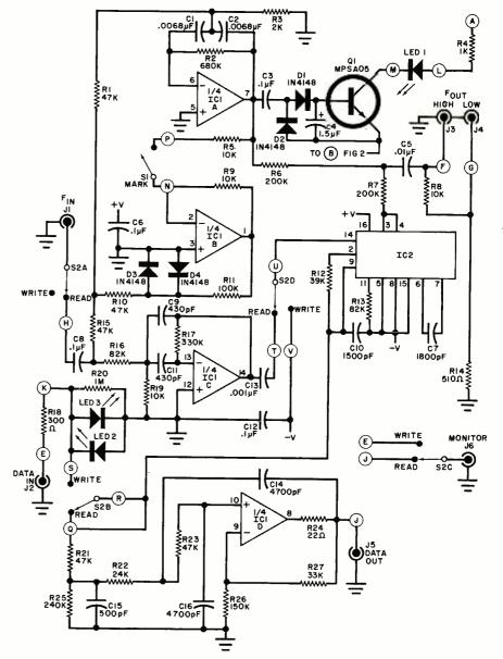
Fig. 2. Schematic of the translator. Letters in circles indicate connections between board and other components.
