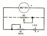
Using a 1.5-volt cell, the resistance of potentiometer R1 should be high enough to limit the current to a safe value. (In this case, a value of 100 kilohms will limit the current to 15  $\mu$ A.) Do not connect R2 at this time. With R1 at full resistance, connect up the circuit. The meter may or may not move upscale. Carefully adjust R1 until the meter goes to full scale. Using a potentiometer of several thousand ohms for R2, set it at full resistance and connect it across a full-scale-
