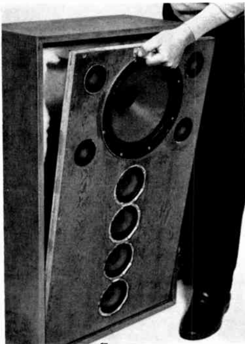
Speaker board must be slowly eased into enclosure to prevent damaging the woofer cone.
