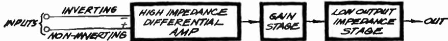
Fig. 1. The basic arrangement of a typical op amp. Such a circuit could contain up to a couple of dozen transistors and associated resistors, all on a very tiny silicon chip.
