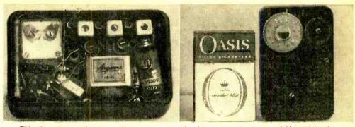
This tiny six-transistor receiver was put together by reader John Jensen of Blair, Nebraska. Note the compact wiring in the interior view at left. The photo at right shows that the finished receiver in its case is not much larger than a pack of cigarettes. See page 125 for details.
