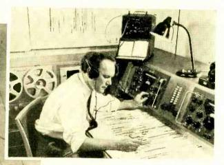
This RFE monitor records the frequency, language, time of day and station of every broadcaster on the short-wave bands. The chart is then used to plot broadcast channels and to locate free channels.
