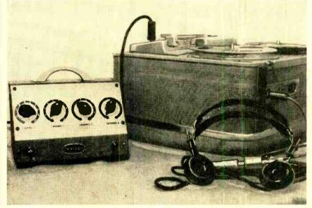
Output of the second recorder feeds into monitor earphones, permitting you to hear previously recorded "tracks" as you add another. Mixer is shown at left.
