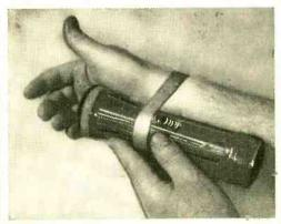
(either standard or penlite size) to your wrist with a wide rubber band. Both hands will be free for work and the light always directed where and when needed. -K. M.
