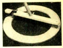
Completely assembled loop, ready for operation. Note terminal strip for connecting the shielded "Twinax" cable, the other end of which connects to a 3-prong plug.
