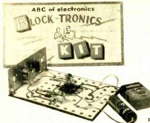
Schematic templates and solderless connections permit fast wiring of many circuits.
