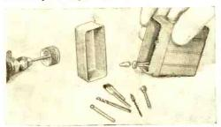
pocket in a plastic cigarette case. Even when hand tool and parts are stored in one larger case, the cigarette container will be convenient. Use as many such containers as are needed. A label, indicating the contents of each container, will speed the work.
