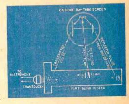
Fig. 4. Pulses of ultrasonic energy are reflected by flaws and displayed on a cathoderay tube. Fig. 5. (below) Illustration of a method for examining odd-shaped metallic pieces for flaws using ultrasonic waves.
