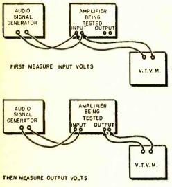
Fig. 3. Method of using an audio signal generator with a vacuum-tube voltmeter to measure amplifier frequency response.
