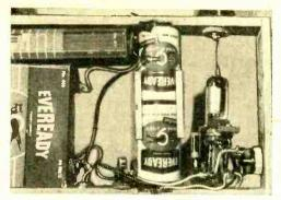
of electronic equipment is to have all of the components available before construction is started. This enables the builder to shift parts around before making any permanent connections. Because it is extremely important to keep all of the leads as short as possible, place the components close to the base of the Vector socket.
