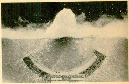
This photo shows the violent agitation of a liquid excited by the curved ultrasonic transducer immersed in the solution.
