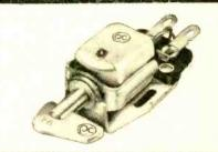
Electro-Sonic cartridges have a frequency range of 20 to 10.000 cycles with a perfectly flat response. The curve then rises gently to about + 1.5 db at 15.000 cycles and 2 db at 20.000 cycles. Output is extremely low, measuring about 1 mv. at an output impedance of 1.5 ohms. The minimum stylus force may be as low as 3 grams. Diamond or sapphire needles are available from the manufacturer.
