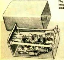
Fig. 2. (Left) The circuit shown in the schematic below (Fig. 3) may be built into an old i.f. transformer can. The resistor chokes and capacitors are mounted on five-point terminal tie strips.
