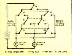
a verbal statement, the circuit must prove the truth of the statement. In this case, the final circuit fulfills the requirements of the man with the upstairs and downstairs halls. In other circuits which can be built with the kit, a similar proof is achieved.
