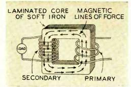
A magnetic field will couple the primary and secondary windings in a transformer.
