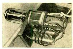
Detailed view of the Vector socket, showing the 27.255 mc. crystal holder made from the terminals of a miniature tube socket.
