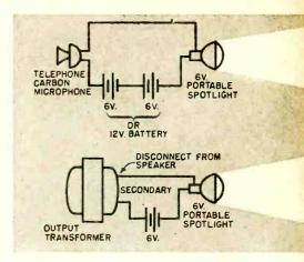
Fig. 1. These two simple transmitters may be used for short-range signaling.
