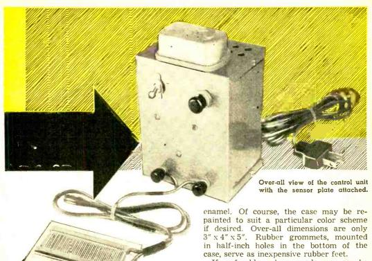
the chassis. Either steel or aluminum may be used, but aluminum is easier to machine and to bend. If steel is used, it will be necessary to give it a protective coating of some sort to prevent rust. Enamel, plastic, or a plating (such as cadmium or copper plating) may be employed.
