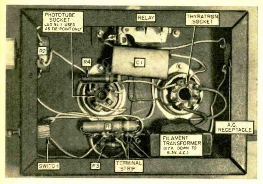
Underchassis view of the control box of the thyratron phototube relay showing the actual placement of parts and wiring details.
