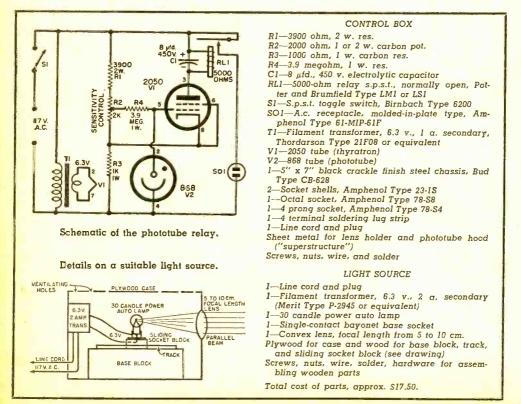
is correctly wired. Assuming that the circuit has been carefully checked after wiring and that all leads terminate at the proper tube pins and tie-points without open or short circuits, certain defects in the components may cause the kinds of troubles listed below. The only instrument required for testing is a vacuum-tube voltmeter having an ohms range or a high-input resistance multitester.
