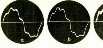
Fig. 5. How frequency response shows up when displaying a sound program on the oscilloscope screen: (a) is the wave presented "flat"; (b) shows high frequency loss; (c) high frequencies over-accentuated; (d) low frequency loss; and (e) low frequencies over-accentuated.
