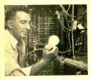
Less power is needed to operate TRADIC than is required to light a 100-watt bulb.
