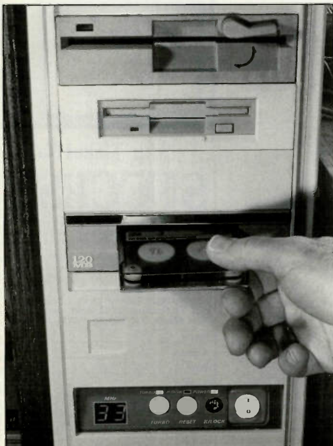
Figure 1. Colorado Memory's Jumbo 120 internal tape drive, installed in a full tower system. The photo shows a tape being inserted. As you can see, the backup physically installs just like a floppy drive.
