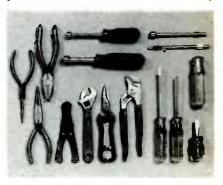
handles; the Series "99" interchangeable screwdriver/nutdriver blades and handles in sets, kits, and individual components; shears; snips; adjustable wrenches; and wire strippers.
