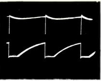
Fig. 8 The output waveform of the tint comparator is greatly different without the VIR. Top trace is the output waveform from the tint comparator in IC60, when VIR control was used. After the VIR was switched off, the waveform resembled a flat-bottomed sawtooth (lower trace).
