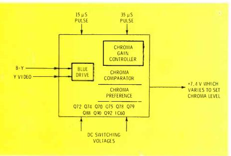
Fig. 9 Except for the input source, the chroma gain controller block diagram resembles that of the tint controller. Blue drive is made by adding video to the B-Y chroma signal. To provide some variation from the correct color level, the color-preference control changes the amplitude of the video that's combined with the B-Y.
