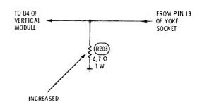
Symptom—Insufficient height Cure—Check R203, and replace if it has increased in resistance
