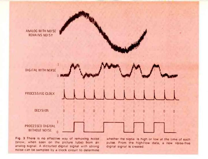
limiters or clippers might remove noise spikes that are much stronger than the signal, but they can't remove any snow.
