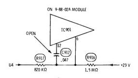
Symptom—Left half of raster is black with three white vertical bars; right half is blacker Cure—Check capacitor C912 on module 9-88, and replace if open
