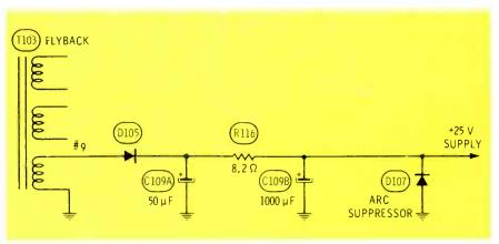
Fig. 7 Power for the +25-volt DC supply comes from the horizontal-sweep pulses at the flyback. When there is no vertical sweep, try the audio volume. A loss of the +25-volt supply will eliminate both. Diode D107 apparently is included as an arc suppressor, clipping off any negative peaks.
