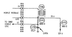
Symptom—No high voltage or 240 V supply Cure—Check capacitor C258, and replace it if open
