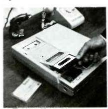
In the "IRC" line, leaders are of heavy-duty (1.5-mil) tape, while "body" tapes are thinner to accommodate long recording times.
