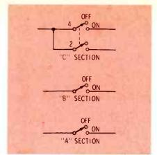
Fig. 9 Some versions of the Admiral M24 and M25 include this "instant play" switch. The "A" and "B" sections open the AC to the bridge rectifiers, when the power switch is turned "off". If one section fails to close in the "on" position, resistor R104 in Figure 2 probably will burn.
