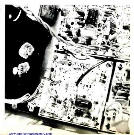
Fig. 2 Four diodes in the main power supply are operated in two different ways. D903 and D902 comprise a full-wave supply, with the B+ taken from the center tap of T100. All four diodes function as a true bridge (the center tap is not used) giving twice the voltage of the other supply. Therefore, overheating of R104 indicates an overload of the +75-volt supply, and not of the +155-volt supply.
