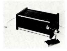
grammed on the coder. When activated by alarm signal, the D8 Dialer will "dial" the programmed phone number and transmit an audible tone code. (If number is busy, dialer will reset and redial until phone is answered.) Then the line stays open for about 1½ minutes so the listener can confirm an intrusion by hearing noises in the protected area.
