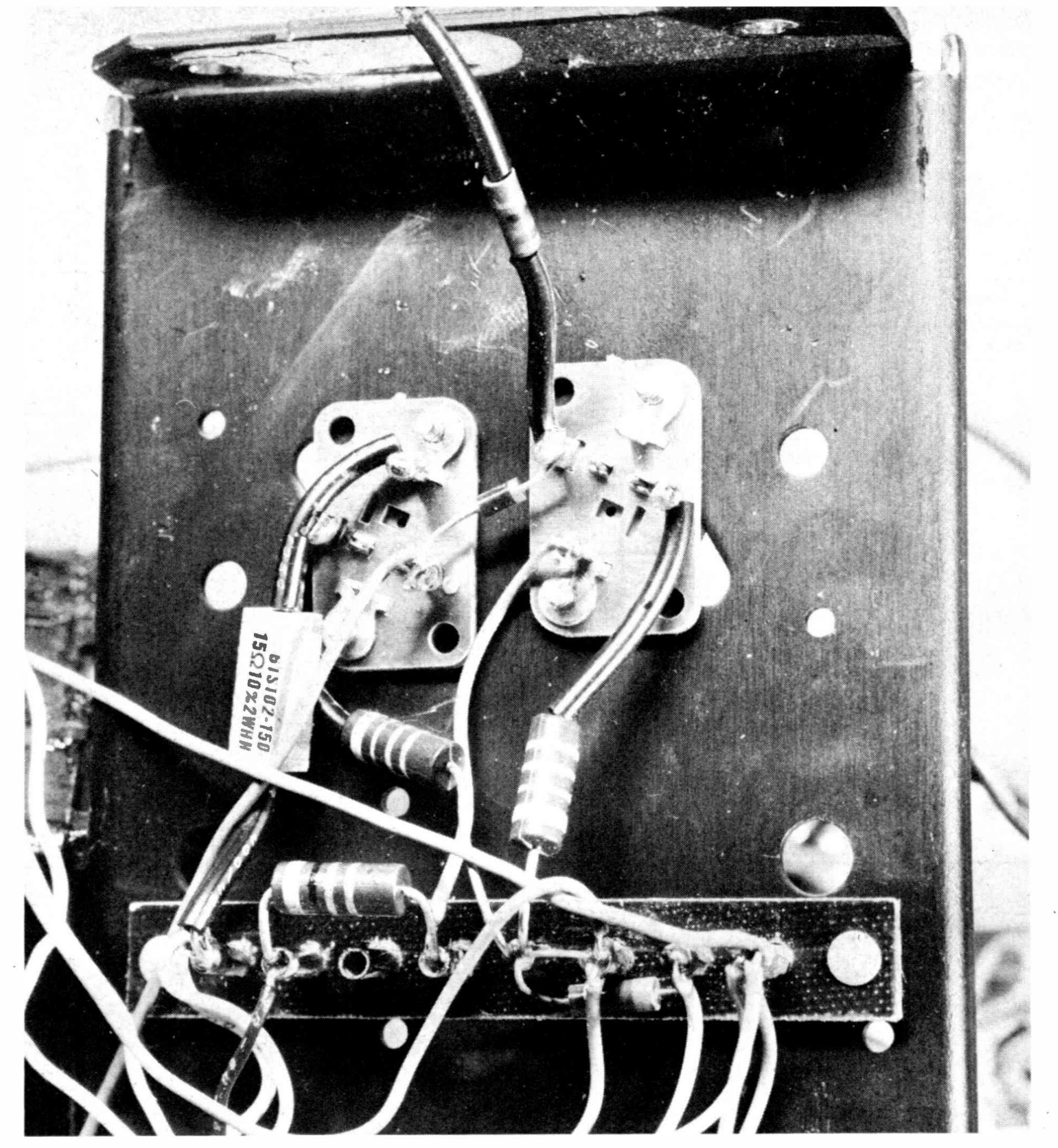
Fig. 4 After you install replacement output transistors, look at the bottom of the sockets to be certain the pins come through the sockets correctly.
