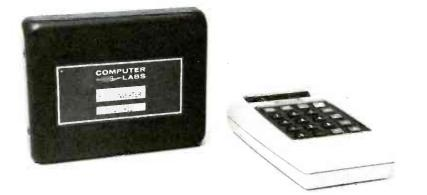
Analog-to-digital converters are not necessarily large. This one by Computer Labs occupies only 21 cubic inches, but it can handle color-TV video with frequencies up to 11 MHz. The price is around \$1,000, but a D/A converter for receivers might cost about \$150. (Courtesy of Computer Labs)
