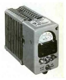
frequency range has been extended to cover 25 to 512 MHz. This adds CB servicing at the low end and land-mobile maintenance at the high end. Load VSWR is 1.1 from DC to 512 MHz and the meter case can be detached for convenient readout. Single unit price is \$249.
