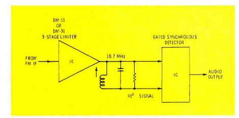
**Fig. 5** Output of the IC with the 3 stages of limiting goes through two paths to the detector; one signal goes direct, and the other is phase shifted by  $90^{\circ}$ . Detection action produces variable-width pulses which are integrated to recover the audio.
