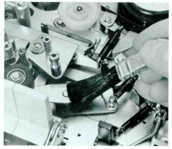
Step 3. Mechanisms are held in the recorder case by screws at the top corners, through the bottom, or at the ends of the cabinet. The handles of portable models generally have to be removed. When you have extracted all mounting screws, carefully turn the machine face down on the soft mat and lift the cabinet off.
