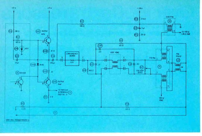
Fig. 2 Output transistors, yoke, and pincushion circuits of the RCA CTC46 chassis.
