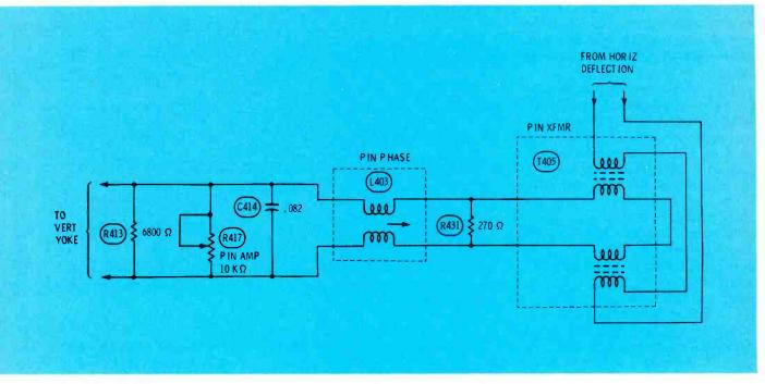
Fig. 3 The RCA CTC58 has one pincushion-correction transformer to accomplish both top-and-bottom and side correction (Photofact 1365-1).
