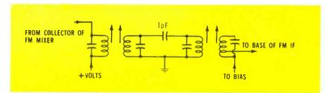
Fig. 2 This quadra-tuned IF circuit provides a curve with flat top and steep side skirts.
