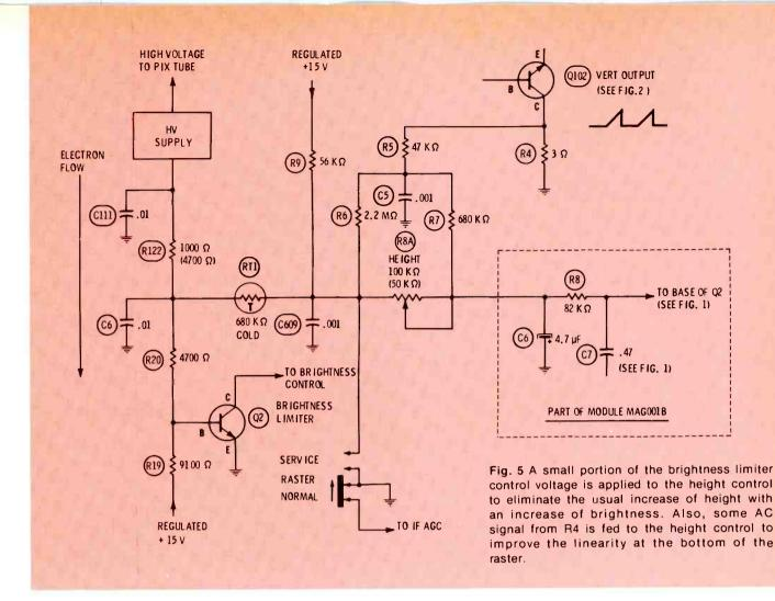
The last input to the heightcontrol circuit comes from the highvoltage system, as shown in Figure 5. Return path from the highvoltage rectifier is to the +15-volt supply via R122, R20, and R19. At the junction of R122 and R20, the voltage varies from near zero with a black raster to a few volts negative at full brightness. A small fraction of this voltage is coupled to the height-control circuit through RT1, which provides temperature compensation.
