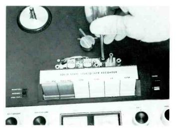
Step 2. Remove the top or front panel. It's usually held by four corner screws. Watch out for screws hidden under the head cover or beneath certain knobs. Carefully work the front panel up and over any control shafts or other protruding parts. Don't try to force it. Most panels are thin metal and bend easily, or plastic that can chip or break.
