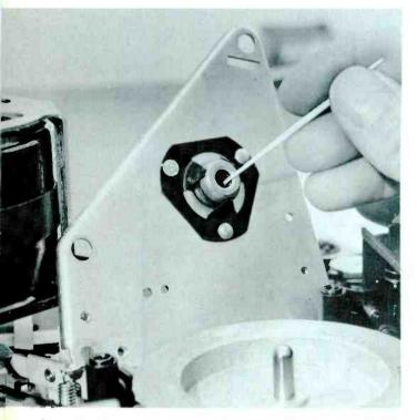
Step 12. After you've cleaned them, lightly lubricate all idler shafts at their bearings. Use a fine silicone grease; oil won't do. Don't overlubricate. Apply a tiny bit of lube to the lower flywheel bearing, too. A toothpick works well for this. Don't use anything metal to apply lubricant. It may score the surface, no matter how slightly, and cause the bearing to wear unduly.
