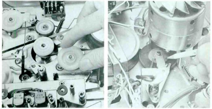
Step 7. Remove all the idlers and give them a good cleaning, especially their rubber rims and their spindle holes. A Q-Tip or other cotton swab is best for the holes. Check the rubber rims for tiny cracks, or spots that are slick or flat. Replace the idler (or the rim, if it's removable) if you can see any defects.
