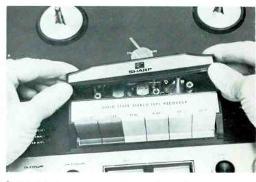
Step 1. All mechanical equipment collects dust, which imbedded in old hardened grease might bind certain moving parts. To get at the parts for cleaning, you'll have to expose the mechanism by removing it from the cabinet. As a first step, remove all control knobs and the head cover. Generally, knobs are push-on types. Grasp them firmly and pull straight up. Avoid tilting the head cover during removal, it's usually plastic, and the mounting posts could break easily.
