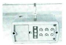
**Fig. 2** In this rear view, the battery compartment is at the left, terminals for external antenna are in the center, and 6 phono sockets for the various signals are at the right.
