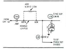
jumper lead from between those lugs, use insulating sleeves on the added resistor, and dress the resistor away from any wire ends on the panel.
