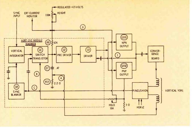
**Fig. 1** Block diagram of the RCA CTC46 chassis (Photofact 1278-3) showing the stages and the feedback loops.
