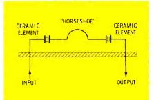
Fig. 4 Ceramic-crystal filters change the 10.7 MHz signal to mechanical motion and then back again to a 10.7 MHz voltage. They give superior curves and don't require tuning in the field. One of the advantages of the PLL decoder is the relative ease of alignment. Usually it is sufficient to adjust to an approximately-correct frequency and let the locking do the rest.
