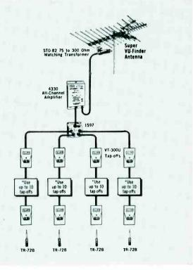
Fig. 1 One example of a "packaged" MATV system. This one handles up to 40 TV receivers.
