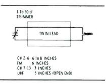
One trap should remove all FM station interference. However, TV stations splatter over a wider bandwidth. So two traps, stagger tuned, might be required to eliminate interference from a strong TV station. Sometimes it is necessary to slide the trap to a different point of the down lead to obtain the maximum effect.
