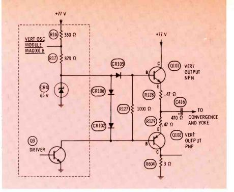
Fig. 4 Some models add two diodes and a resistor between the bases of the two output transistors.
