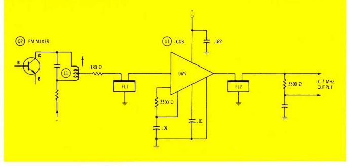
Fig. 3 An IC Gain Block (ICGB) includes two ceramic filters and one IC.
