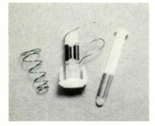
Fig. 3 A fine tuning coil used in older RCA tuners. The tip of the plunger contains inserts of powdered iron. Often the iron inserts fall out or break and either jam the movement or cause inadequate fine-tuning action. Buy a new coil and cross-switch the two cores. This eliminates the need for adjusting each channel screw or replacement of the coil.
