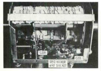
Remove several coil strips to make room for "live" testing. Strips are coded with numbers and colored dots. Capacitors C220 and C221 are the most critical components in the oscillator circuit.
