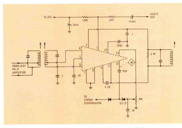
Fig. 9 Quadrature detector circuits, such as this one, used in Delco AM/FM stereo radio Model 02GFP1, require an alignment procedure which is different than that used with receivers equipped with conventional detectors. See text for detailed procedure.
