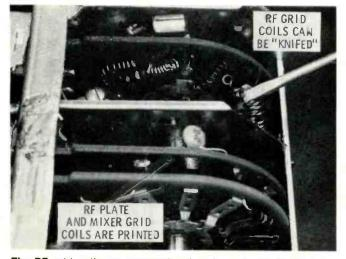
The RF grid coils are conventional and can be "knifed" during sweep alignment. The RF plate and mixer-grid coils are "printed" on the board and cannot be adjusted.
