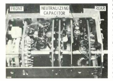
Location of the neutralizing capacitor. To perform neutralization: 1) bias the 6DS4 to cutoff by applying -15 volts or more to the tuner AGC point; 2) tune in a highband station, preferably on channels 8, 9 or 10; 3) adjust neutralizing capacitor for minimum video. Use a nonmetallic screwdriver.
