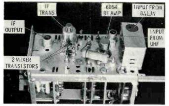
KRK144A hybrid tuner used in late-model RCA color receivers. The balun coil is mounted, with the antenna terminal strips, on the cabinet back. The tuner is very small, but accessibility is good.
