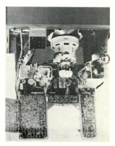
rails, it also can be slid out, for improved accessibility of components on the front of the chassis. Removal of five screws releases the cabinet rear cover. The bottom of the cabinet also can be removed, to provide access to the bottom of the chassis without sliding out the chassis.
