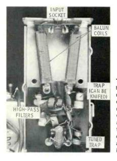
The balun coils can be damaged by lightning or static discharges. Be sure the relative phase of the windings of new coils are correct. The IF trap that has a core can be mistuned to an interfering signal in the 40-MHz range.
