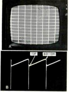
Fig. 2 Normal raster and normal waveform produced by yoke voltage, for purposes of comparison. (A) Normal raster with crosshatch pattern displayed. (B) Normal voltage waveform applied to the vertical windings of the yoke.
