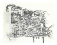
Signal-processing circuit board of U-1 chassis, shown here, contains video IF and amplifier stages, AGC circuitry, the horizontal oscillator and buffer, and the vertical oscillator and buffer. Component adjustment and test point callouts and circuit pattern are printed on both top and bottom of board. Note that all connections to board are plug or slip-on type; unsoldering and resoldering are not required to remove or re-install board.
