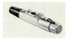
No. T(\*)F has a black neoprene strain relief and accepts cables up to 0.25-inch in diameter; T(\*)FL has the same type of strain relief, with a larger cable opening to accomodate cables from 0.25-inch to 0.328-inch in diameter.
