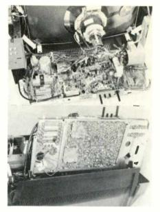
Main chassis of U-1-equipped receivers slides back on two tracks, to completely expose all circuitry, adjustments and test points on the top and the bottom of the chassis, as shown here. Chassis is freed from normal operating position by releasing two clip-type, retainers, pointed out by large, white arrows in top photo. Note that components and test points are labeled both on the top and on the bottom of the signal-processing circuit board.
