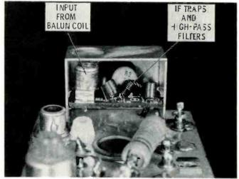
Shielded box at rear of the tuner contains the input plug for the shielded cable from the balun coils, and the traps and high-pass filters.
