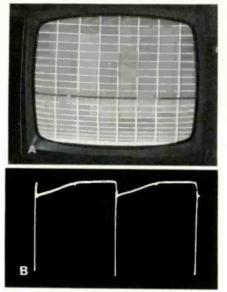
Fig. 5 Two complete pictures caused by vertical sweep at 30 Hz. (A) Crosshatch reveals two pictures, with the bottom one compressed. (B) Distorted yoke waveform and one sweep pulse for each two sync pulses are produced when sweep frequency is 30 Hz.
