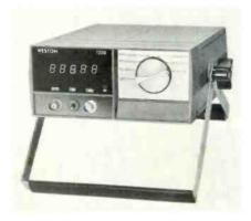
Time Base Stability-±10 PPM/ 10 degrees (C) to 40 degrees (C), Ref. temperature of 25 degrees
