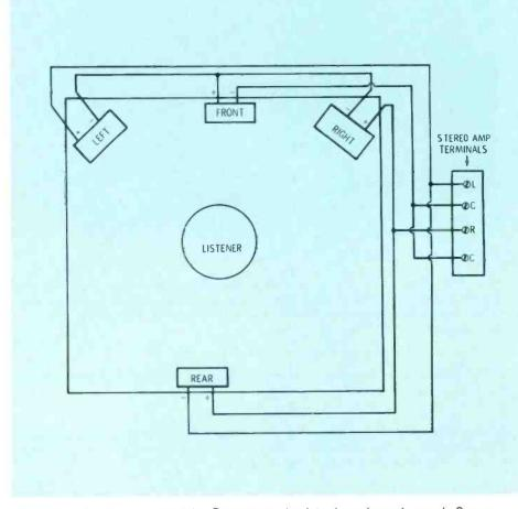
Fig. 5 Speaker hookup used by Dynaco to simulate four-channel sound. Separations among various speakers are enhanced by recordings made for this setup (Brothers Records, Los Angeles).
