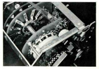
Stator switch wiping contacts can cause loss of all stations, if they become bent. Older models were prone to intermittents caused by loose rivets. The cure is to solder them to the switch.
