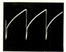
Fig. 8 Waveform produced at the vertical output transformer when the yoke is disconnected shows more non-linear sawtooth and significantly less pulse. This pulse is caused by the collapsing magnetic field of the vertical output transformer.
