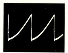
Fig. 7 Waveform produced by normal cathode current in the vertical output tube. Most of the large, negative-going pulse, which is at the grid, occurs after the tube is cut off, and the pulse does not appear at the plate or in the plate-cathode current.
