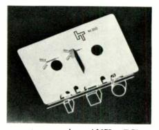
cassettes meeting ANSI, ECMA and audio standards, according to the manufacturer. It is placed in the drive in the same manner a cassette is inserted, and the machine then is set to the "play" mode. A separate reference block, machined to the width of a cassette tape, is placed on the gauge to provide an accurate reference for positioning drive components.
