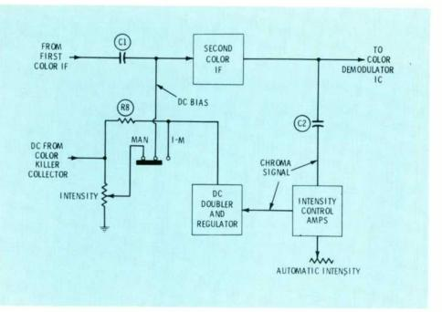
Fig. 2 Automatic color-intensity circuit is one of the functions brought into play by pushing Insta-Matic button. Pre-set contrast, brightness, hue, and color controls are also activated, plus a circuit that desensitizes the color demodulator to flesh color variations and adds a slight red shade to the raster.
