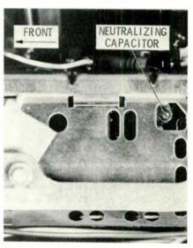
Fig. 2 Location of the neutralizing capacitor on the left side of most RCA tuners. It can be adjusted without removing the shields.
