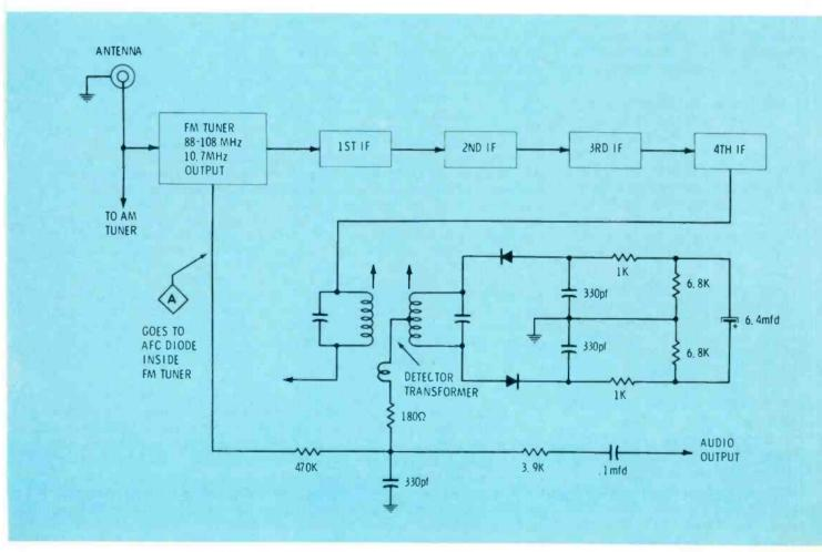
Fig. 4 Simplified block diagram of a typical FM receiver (Motorola Model FM991).
