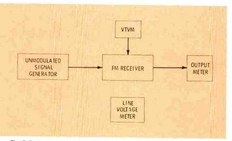
Fig. 7 Equipment setup for performing non-swept alignment of most types of FM receivers. See text for detailed procedure.
