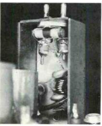
Twin-lead connects the antenna terminals on the cabinet back to the two tuner input prongs, which are also feedthrough capacitors for isolation of the antenna circuit from the "hot" chassis. The balun coil is mounted next to the feedthroughs; the coils and capacitors below it are the high-pass filter assembly.
