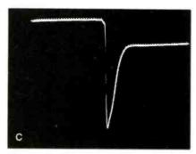
Fig. 10 The pulse portion of the yoke voltage waveform (widened 5X), with different types of loading across the yoke. (A) Normal voltage pulse at the yoke. Notice the horizontal pulses "riding" on the waveform. (B) Increased ringing caused by increasing C39 from the normal .1 to .6 mfd. Most of the horizontal pulses have been by-passed. (C) This loss of normal overshoot is caused by adding a 820-ohm resistor in parallel with the yoke.
