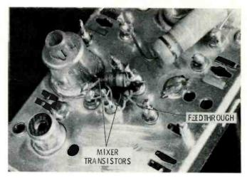
Two cascaded mixer transistors are mounted on feedthrough capacitors.
