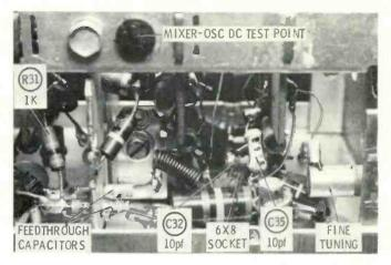
Capacitors C32 and C35 are likely suspects if all stations tune in one or more channels below normal. R31 (1000 ohms) will burn and its value will change when the 6BQ7 shorts; test it, because the value affects the proformance of the RF amplifier.
