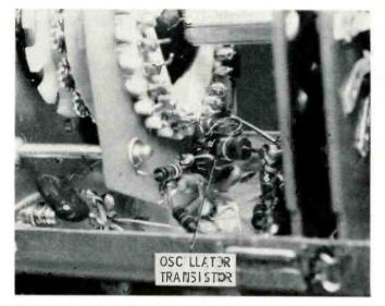
Oscillator transistor is mounted on the rear side of the oscillator switch-stator board.
