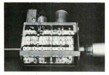
The tuner used in Silvertone chassis 456/528, 51780 is a turret type with plug-in strips.
