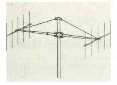
telescopic design permits them to be extended to optimum spacing, according to the manufacturer.
