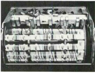
Stator contacts before and after cleaning. Several strips have been removed to provide access. Upper-dirty; lower-clean.
