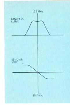
Fig. 5 Typical response curves produced by properly tuned FM receiver.
