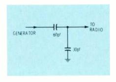
Fig. 6 Circuitry of a dummy antenna which can be used between the signal generator output and the signal injection point of most auto FM receivers.
