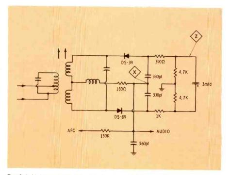
Fig. 8 A high-impedance DC voltmeter, connected to point Z in the demodulator circuitry shown here, serves as the indicator during non-swept alignment.
