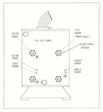
Color saturation produced in "on" position of AccuMatic control not the same as that in "off" position **RCA CTC46**
