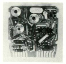
Fig. 3 AccuCircuit plug-in module cards are major design features of new RCA chassis CTC 46 and CTC 54. Five integrated circuits are used. Now-standard SCR horizontal deflection is retained in these new chassis.
