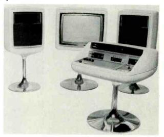
Futuristic home entertainment complex from Panasonic contains AM, FM stereo, 8-track stereo tape, and color television, all controlled from special console in foreground. Digital timer turns system on or off. Tiny 2-inch b-w monitor in console can be switched to any channel for preview before changing the program on large center screen. This is prototype, but suggests future designs.
