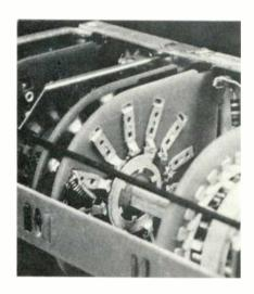
Fig. 1 One type of tuner switch contacts consist of double stationary wiping contacts made of spring material, and a knife contact that slides between. The contacts shown here are clean.
