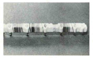
The two strip contacts on the left have been cleaned; the three on the right are still corroded. Use a cloth and a degreasing liquid to clean such contacts.
