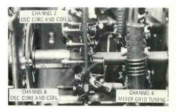
All the coils are electrically in series, starting with channel 13. If the oscillator will not adjust to the correct frequency on one channel, adjustment of the channel above it might be necessary. The low-band oscillator coils can be "knifed", if necessary to obtain the correct frequency.
