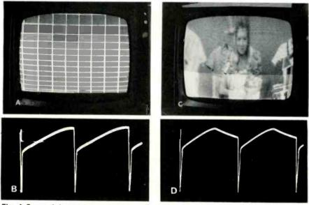
Fig. 4 Some defects cause stretching at top and compression at bottom. (A) Crosshatch pattern when the height control is too low and the linearity control adjusted too high. (B) Waveform when the height control is too low and the linearity control adjusted too high. (C) Leaky C34 caused extreme stretching at the top and foldover at the bottom. (D) Yoke waveform produced when C34 caused bottom foldover.
