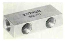
The splice block, Model SS/U, is designed for RF coaxial transmission systems and CATV systems operating in the frequency range of 5 MHz to 230 MHz and 26 dB up to 300 MHz. The unit measures  $1\frac{1}{4}$  inches x  $\frac{3}{4}$  inches x 3 inches and has standard  $\frac{5}{8}$ -24 entry ports. It is housed in corrosion-resistant aluminum.
