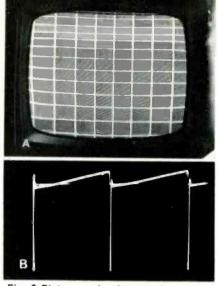
Fig. 3 Picture and yoke waveform when the height control is adjusted too high and the linearity is adjusted too low. (A) Raster with a crosshatch pattern which reveals compression at the top. (B) Yoke waveform, which produced compression, is flattened at the start of the sawtooth.
