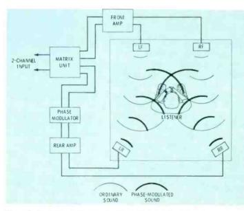
Fig. 13 Function diagram of method used by Sansui to synthesize what sounds like surround audio under some listening conditions. Synthesizer can be added to existing system.
