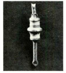
Fig. 4 One type of feedthrough capacitors used in tuners. The two white bands are ceramic insulation; the flange in the center is soldered to the chassis of the tuner. Avoid solder splatters.
