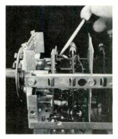
Fig. 5 When it is necessary to cut a wire, but the diagonal cutters won't reach, use a two-pronged soldering aid to break the wire by bending it back and forth.
