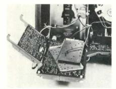
The IF circuit panel is shown here in the swing-out position. During normal operation, the panel is covered with metal shields, shown here removed. Normal adjustments can be made through the shields, if required. The circuitry on the IF panel, as on all panels, is "road-mapped" on both sides, for easy component and circuit identification. Note the plastic press-fit buttons, on corners of panel, which hold chassis in vertical position during normal operation.
