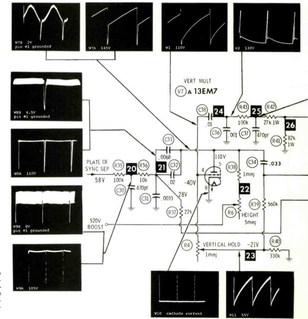
Fig. 1 Complete schematic diagram of the vertical sweep system in Sears' 528.-51780 b-w chassis. The voltage at the plate of the output tube normally should change only about 20 or 30 volts regardless of height and linearity adjustments, and not much more than that after most defects.
