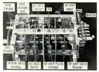
**KRK22 tuner** used in an RCA CTC5 chassis is a "switch" type and employs a 6BQ7 RF amplifier tube in a "cascode" circuit which requires no neutralization.
