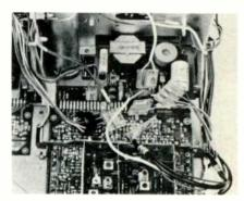
**Quick-disconnect** plugs, some of which are shown here, are used throughout the CS-195 receiver, to eliminate the need for soldering and resoldering of wiring for removal and installation of the circuit boards and panels which make up the chassis. Again, note the clear road mapping of circuitry and identification of components and test points.
