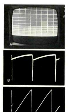
Fig. 6 Picture and waveforms produced when C3C cathode bypass is open. (A) Compression and loss of height at the bottom is produced by open C3C. (B) Yoke waveform reveals flattening at the top of the sawtooth. (C) Waveform with amplitude of 34 V PP is produced at the cathode when C3C is open.
