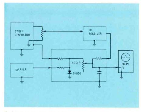
Fig. 3 Typical setups for performing sweep alignment of an FM receiver. See text for detailed procedure.
