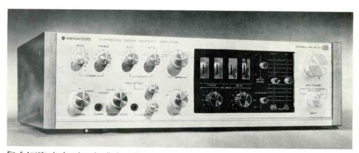
Fig. 6 Amplifier for four-channel audio has built-in reverb to emphasize big-hall sound. (Label "Hall Effect" does not refer to the well-known magnetic effect.) Slider controls set balance between front and rear speakers. VU meters are provided for all four channels.
