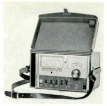
Accuracy of the Model 747 is  $\pm 1.75$  dB, 50 to 260 MHz; and  $\pm 3$  dB, 470 to 890 MHz, over a temperature range from 20 degrees (F) to 100 degrees (F). The unit provides simultaneous readings in microvolts and dBmV, with a range from 10  $\mu$ V (-30 dBmV) to 1.0 volts (+60 dBmV), according to the manufacturer.
