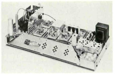
Fig. 4 New Zenith all-solid-state color chassis, the 25CC55, didn't make the CES but was shown nearby at the company's Chicago showroom. Newest addition is thick-film integrated circuit that develops horizontal sweep (but not output).
