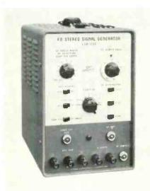
The new unit not only checks separation and balance in FM receivers and tuners but also reportedly serves as a sweepmarker for 10.75 MHz FM and IF alignments.
