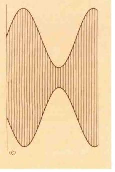
Fig. 1 Elements of amplitude modulation. A) Unmodulated carrier. B) Modulating signal. C) Amplitude modulated carrier. All of these can be viewed on a scope. One of the persistent fears that prevents some technicians from realizing the most from FM radio servicing is alignophobia. This is characterized by a fear of touching tuned circuits above 2 MHz or so.
