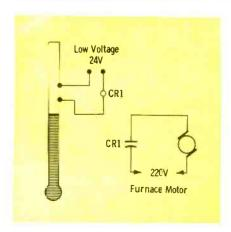
Fig. 1. Basic construction of a mercury temperature switch used to actuate a furnace control relay.
