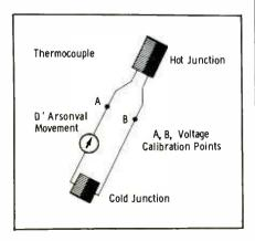
Fig. 6. Structure of a thermocouple.
