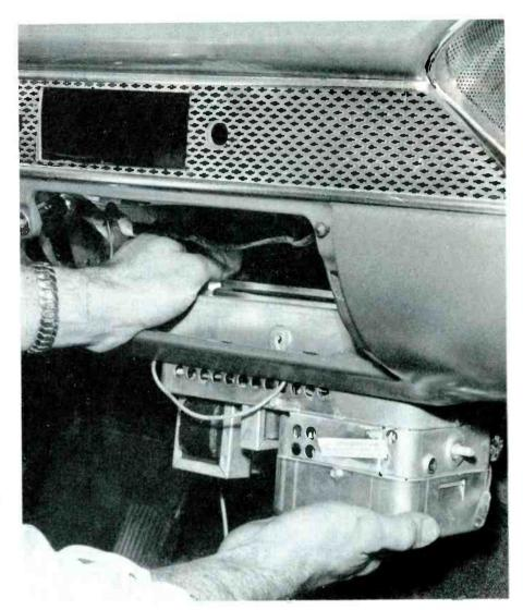
Fig. 2. Removing chassis.
