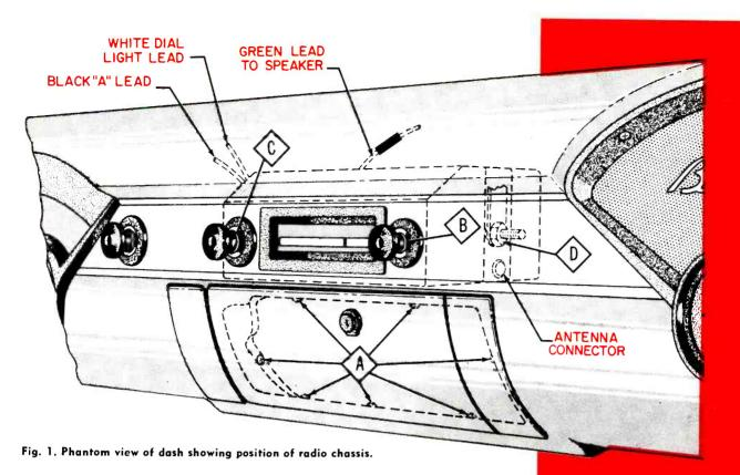
Removing an auto radio is basically more a physical task than anything else; however, it is one which can require some time and effort due to the awkward position in which the technician has to place himself in order to reach the screws, nuts and bolts under the dash panel. A knowledge of the correct procedure and the exact tools for removing radios in specific makes of cars will help to reduce the time and effort involved in these tasks.
