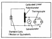
Fig. 7. A portable potentiometer connected across a thermocouple unit can be used in conjunction with a chart to determine temperature of the hot junction.
