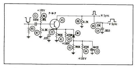
Fig. 3. A one-stage sync separator using a diode-controlled time constant.
