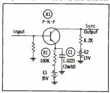
Fig. 2. A single-stage sync separator.
