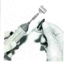
Fig. 2. Attachments for Win-Tronix intermittent probe pemit signal sampling without direct circuit contact.
