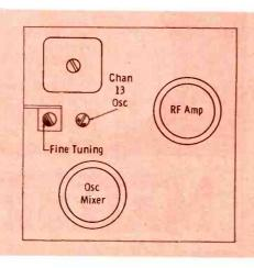
Fig. 3. Channel 13 oscillator adjustment on top of tuner.
