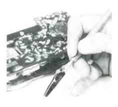
Fig. 2. A needle-point probe is ideal for transistor-radio testing.
