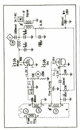
Fig. 2. Mixer and oscillator section of turret-type cuner.
