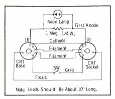
Fig. 2. CRT emission indicator which utilizes a meon lamp shunted by a 1-meg resistor in the first-anode lead.
