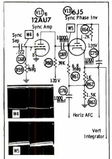
Fig. 3. Intermediate sync amplifier with grid input—Fada Model H274T.
