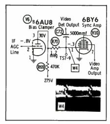
Fig. 6. Bias clamper for pentagrid separator—General Electric "ST" Line chassis.
