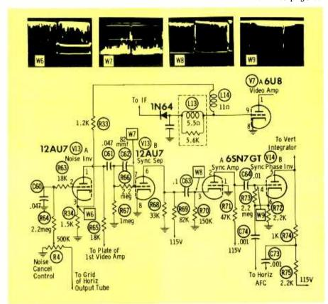
Fig. 2. Sync section plus triode noise inverter—Stromberg-Carlson Model 621.
