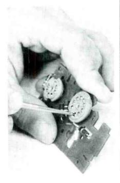
Fig. 3. Using a soldering aid to tighten
