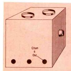
Fig. 2. Left side of RCA Tuner showing location of channel 6 adjustment.
