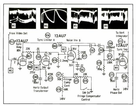
Fig. 4. Sync preamplifier and keyed noise inverter—Emerson Model 748B.
