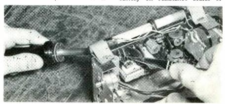
Fig. 8. Use of a heat sink is very important when soldering transistor leads.
