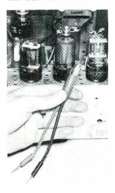
Fig. 1. Neon test lamp being used to check for the presence of oscillator energy at the horizontal output tube.
