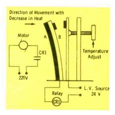
Fig. 2. The contacts of a bi-metal thermostat will open and close over a predetermined temperature range of 2° to 3°F.
