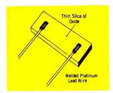
Fig. 3. Simple sketch of a thermistor.
