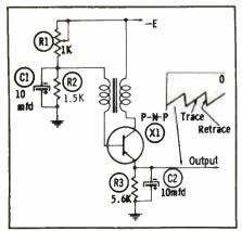
Fig. 5. Development of the sawtooth wave in this circuit differs from Fig. 4.
