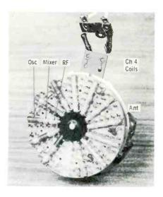
Fig. 2. Bottom view of new tuner showing tuner coils mounted on wheel.
