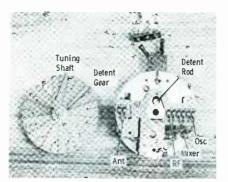
Fig. 3. Wheel removed to show contacts.
