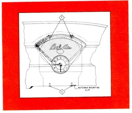
Fig. 3. Phantom view showing position of speaker unit.
