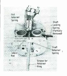
Fig. 4. Components which must be loosened or removed to free the coil wheel.
