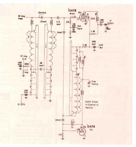
Fig. 1. Mixer and oscillator section of switch-type tuner.
