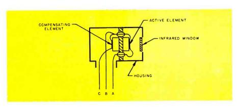
Fig. 4. Internal makeup of a bolometer.
