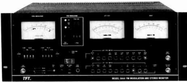
Figure 2. A combined frequency and modulation monitor. (Courtesy TFT, Inc.)
