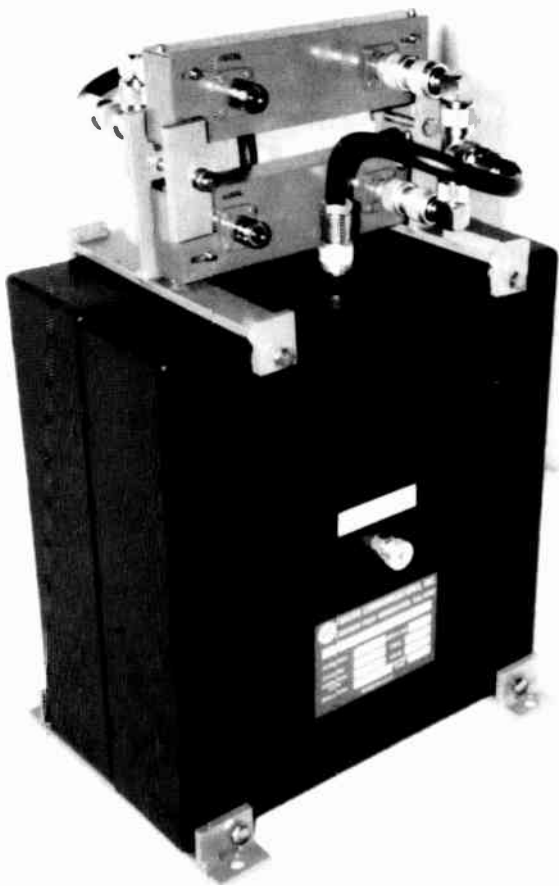
Figure 21. UHF low-power TV notch diplexer. (Courtesy Micro Communications, Inc.)
