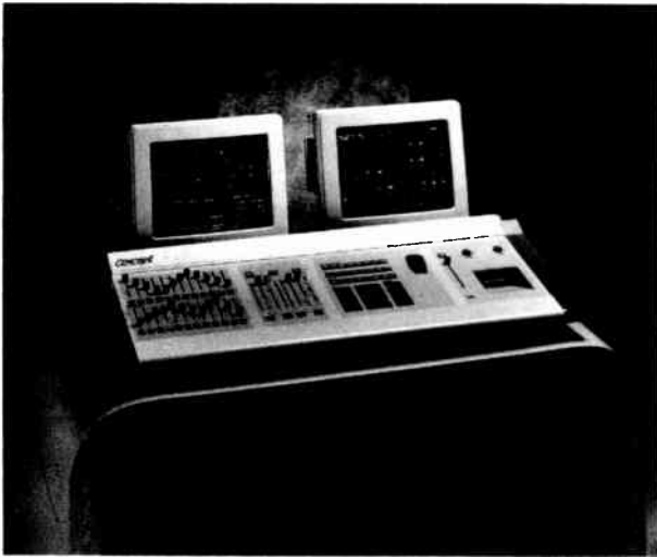
Figure 31. The most sophisticated consoles utilize dual CRT displays and can control very large quantities of dimmers with equal number of discrete channels.
