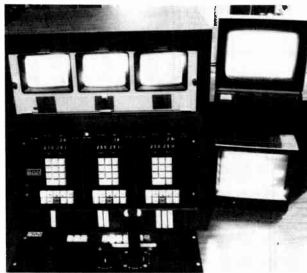
Figure 1. A custom-made console is equipped with monitors for the cameras, program line output, and teleprompter.
