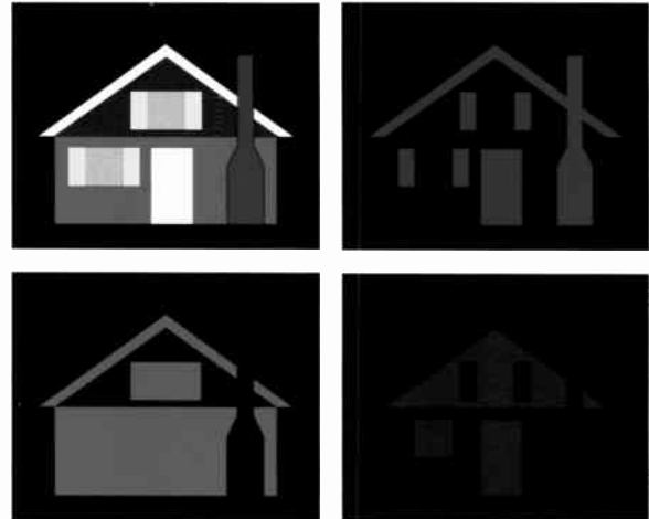
Figure 10. Illustrating how a typical color image (upper left corner) can be separated by optical means into red, green, and blue counterparts.
