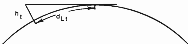
Figure 6. Distance to radio horizon.
