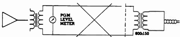
Figure 2. DON'T meter the signal across the input to the repeat coil (transformer at right) and DON'T feed the repeat coil directly from another transformer, if possible.
