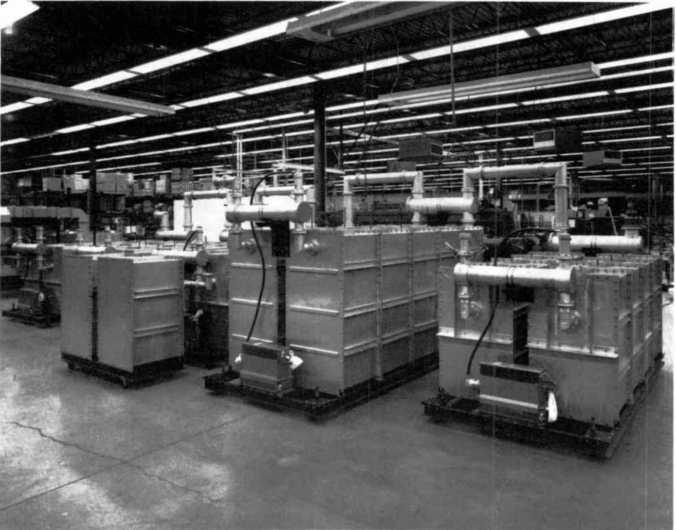
Figure 18. Four-channel multiplexer: Ch. 6, plus three FM's. Corpus Christi, Texas.
