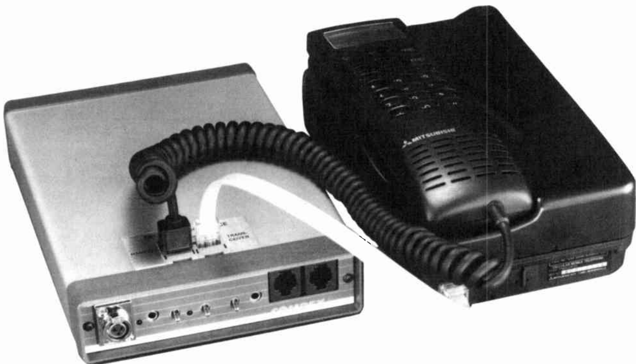
Figure 10. Interface to cellular telephone for broadcast on-air use. (Courtesy Comrex.)
