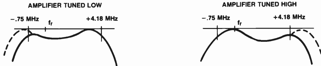
Figure 61. Nonsymmetrical response caused by the amplifiers outside the transmitters bandpass. Solid line is transmitter overall response. Dotted line is the part of PA response outside of the transmitters bandpass.
