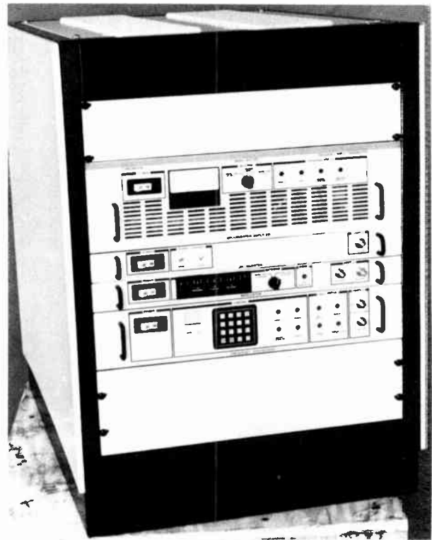
Figure 10. ITFS/MMDS frequency agile transmitter.
