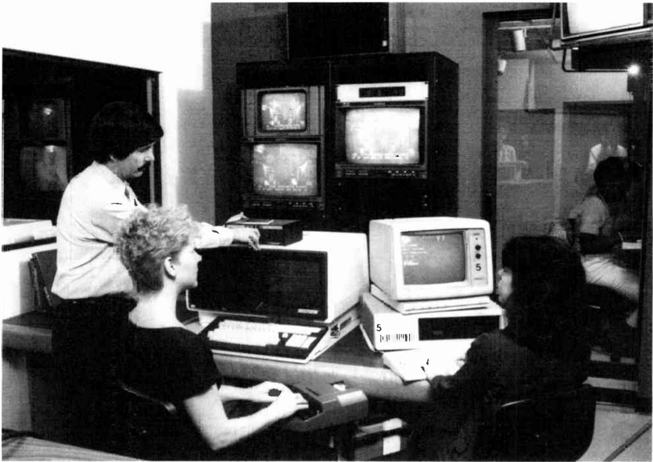
Figure 6. Real-time captioning is done by an operator using a stenotype keyboard similar to those used by court reporters. (Courtesy of National Captioning Institute.)
