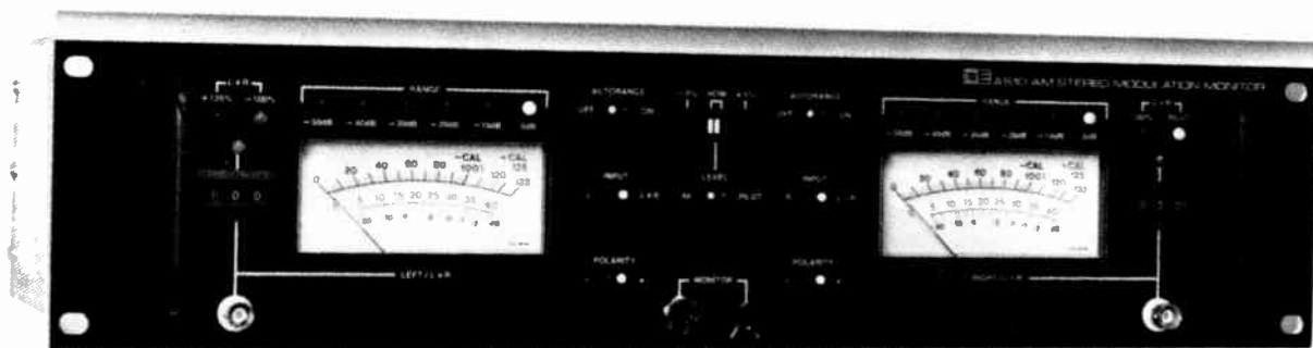
Figure 13. Broadcast Electronics Model AS-10 C-Quam AM stereo modulation monitor.
