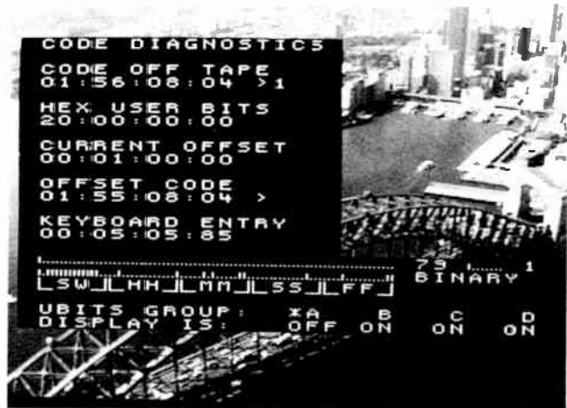
Figure 13. ADX-02 timecode analyzer diagnostic. (Courtesy ADX)
