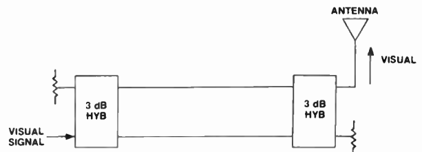
Figure 87B. Visual signal applied to back-to-back hybrids.
