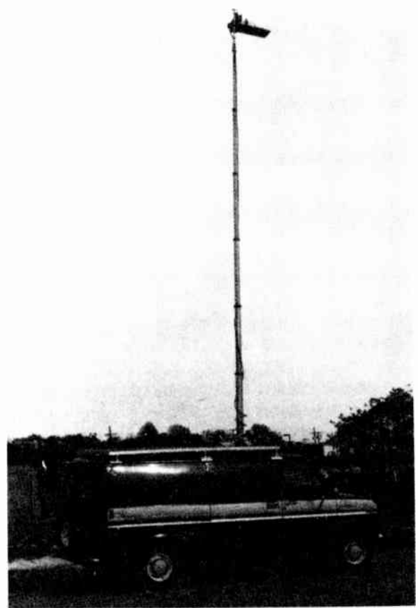
Figure 9. Van equipped for making field strength measurements with 30 foot antenna height.
