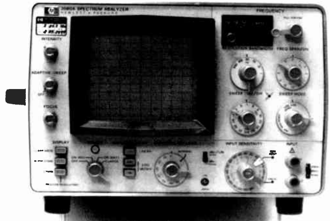
Figure 6. Spectrum analyzer intended for audio use.
