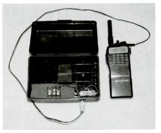
ally because their terminals line up along the right wall of the recipe box. The jumpers are clipped, not soldered, to the terminal tabs so you can replace packs singly if needed.
