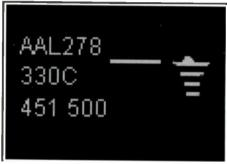
This is an example of how a data block might look on a radar screen. It shows AAL278 (American Airlines Flight 278), 330C (Mode C, Flight Level 330), 451 (Computer ID number), 500 (Ground speed). The horizontal line points to the aircraft on the right, a dot. The tapering lines indicate northbound travel / up on the screen. Courtesy: NASA Ames Education Division
