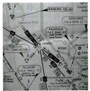
This is the LANDO intersection on the IFR ENROUTE HIGH ALTITUDE H-2 Chart. Note the Jet Routes J5, J6, J50, and J65 passing through this intersection.
