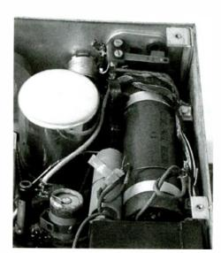
Cobbled-up replacement of multisection filter cap in original radio. Factory capacitor, abandoned in place, is large cylindrical unit at right.
