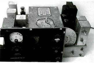
Original radio with cabinet and panel removed. Note warped section of bandspread dial (to right of panel top corner) and resistors wired into dial lamp circuit.
