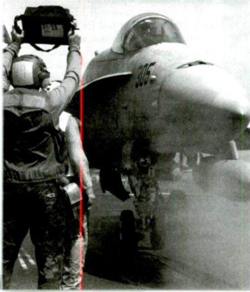
Aviation Boatswain's Mate holds up a weight board firming the weight of the aircraft to be launched on USS Kitty Hawk (CV 63). Kitty Hawk demonstrates power projection and sea control, as the world's permanently forward-deployed aircraft carrier, based in Yokosuka, Japan. (U.S. Navy photo by Photographer's Mate Airman Bo J. Flannigan)
