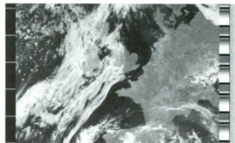
Fig 1: NOAA-17 September 4, 1116UTC visible-light channel showing minute marker intervals on the left side and the calibration wedge blocks on the right, with the tone-burst signal on the far-right edge.
