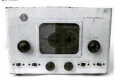
Circuitry: a.c.-d.c. superhet (no power transformer). No r.f. stage; one i.f. stage; bandspread; built-in speaker; BFO. Tube complement: 12SA7 oscillator/mixer; 12SK7 i.f. amplifier; 12SQ7 detector, AVC, first audio amplifier; 12SQ7 BFO; 35L6 audio output; 35Z5 rectifier.
