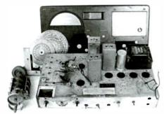
Virtually bare S-40 chassis as stripped down for refinishing. Capacitor can to left of transformer will be removed after replacement below the chassis, then reinstalled – just for looks – -after paintwork is completed.
