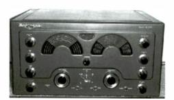
bration every 50 kHz on the range 1.6 to 4.4 MHz, every 100 kHz from 4.4 to 12 MHz and every 200 kHz from 12 to 31 MHz. There is a separate bandspread (fine-tuning) knob with a dial scale calibrated for the ham bands. Unlike cheaper sets of the time which used backlash prone dial cord to couple the tuning knob to the tuning dials and tuning capacitors, the 183D used a smooth geared dial drive.
