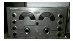
Reception modes were AM and CW via a variable BFO – there was no product detector since SSB hadn't come into wide use at the time. A plug-in adapter for narrow band FM was an optional accessory. A separate speaker or headphones are required, since there is no internal speaker. The radio sold new for \$399, according to an ad in the 1956 Amateur's Radio Handbook. Fred Osterman's book Shortwave Receivers Past and Present lists a used price range of \$150 to \$290 for the radio.
