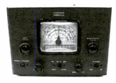
Circuitry: a.c.-d.c. superhet (no power transformer). No r.f. stage; one i.f. stage; bandspread; built-in speaker; BFO. Tube complement: 12K8 oscillator/mixer: 12SK7 i.f. amplifier; 12SQ7 detector, AVC, first audio amplifier; 12J5 BFO; 35L6 audio output; 35Z5 rectifier.
