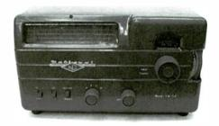
Circuitry: a.c.-d.c. superhet (no power transformer). No r.f. stage; one i.f. stage; thumbwheel tuning aid, but no bandspread; built-in speaker; BFO. Tube complement: 12BE6 oscillator/ mixer; 12BA6 i.f. amplifier/BFO; 12AV6 detector, AVC, first audio amplifier; 50C5 audio output; 35Z5 rectifier.
