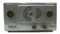
Circuitry: a.c.-d.c. superhet (no power transformer). No r.f. stage; one i.f. stage; bandspread; built-in speaker; BFO. Tube complement: 12SA7 oscillator/mixer; 12SK7 i.f. amplifier/ BFO; 12SQ7 detector, AVC, first audio amplifier; 35L6 audio output; 35Z5 rectifier.
