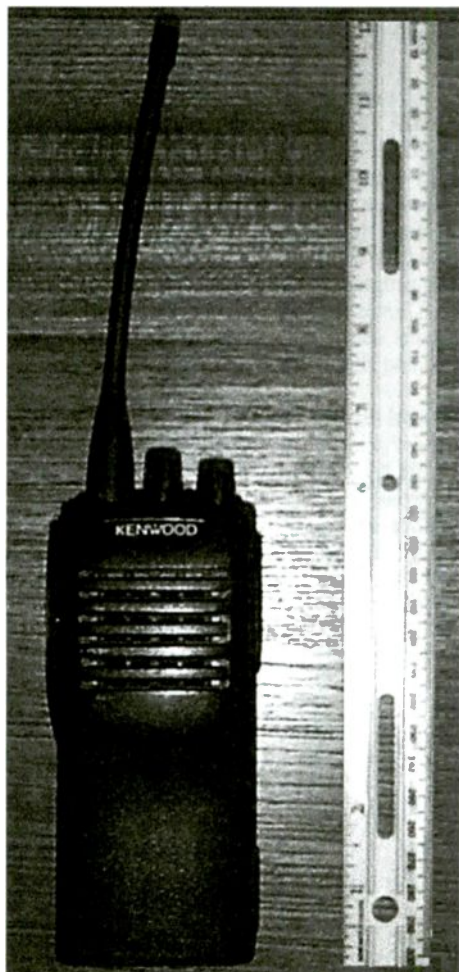
The Kenwood TK-360 is a four-channel conventional radio operating in the VHF band.
