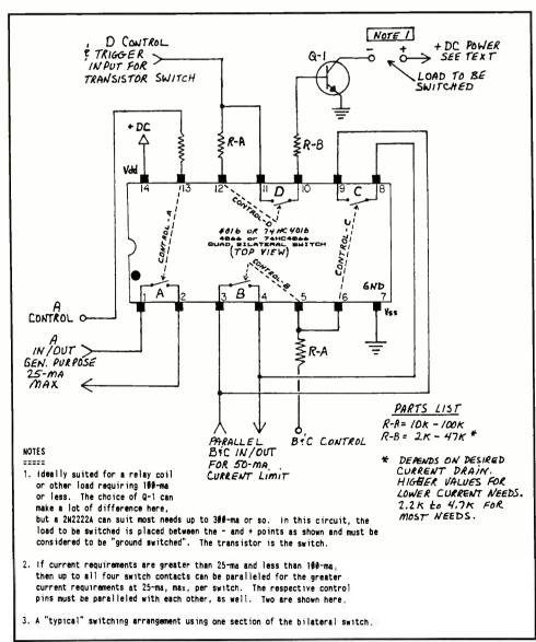
Figure 1: Typical Applications for a Bilateral Switch
