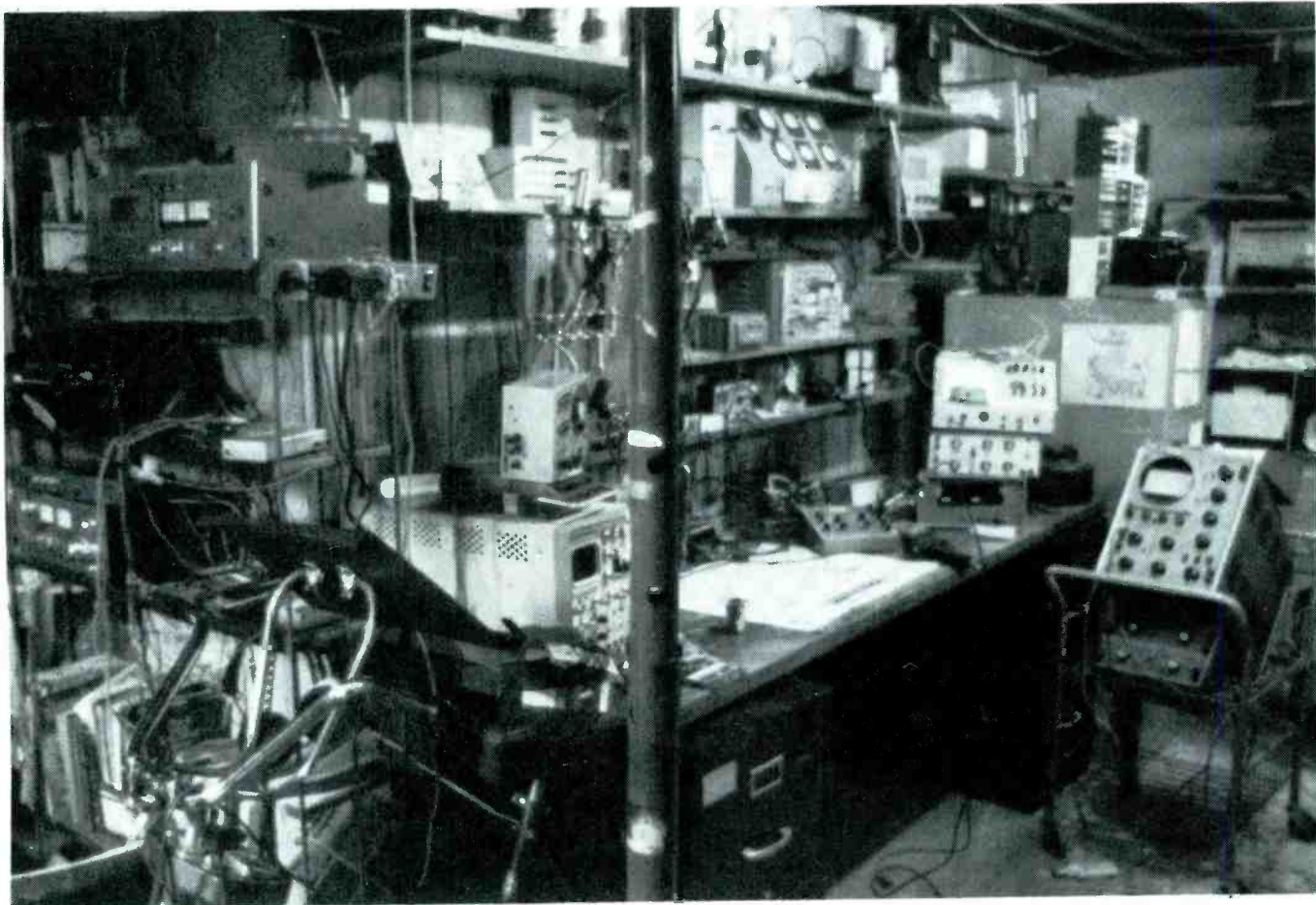
A view of the workshop used by the author. On the wall near the center of the picture can be seen an equipment power box with built-in switch. Separate switches and fuses are provided for lights and test equipment. Equipment on shelves and racks are securely mounted so that they can not be pulled off by their test leads.
