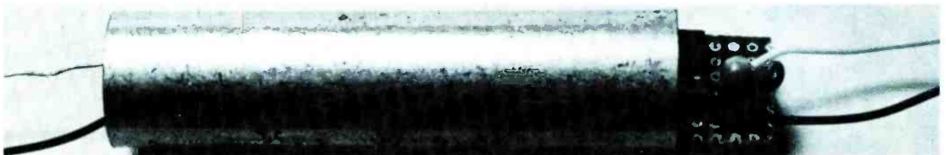
THE PROBE'S PARTS are small enough to mount on a perboard that is 7/16-inch wide. The board's length is not critical. There's sufficient space inside most probes to permit mounting of parts. Refer to text for shielding information.
