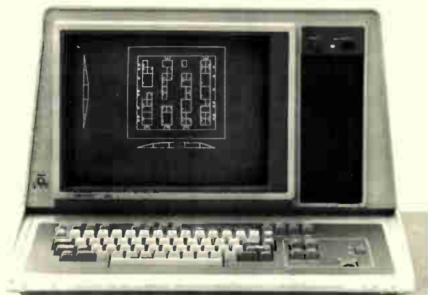
2. Graphics terminal. The LDS I uses a Tektronix 4112 or 4113 graphics terminal as its interface with the designer. The terminal's power greatly enhances the total system. It uses a 16-bit 8086 with 500-K bytes of memory and a floppy disk, and it is programmable.
