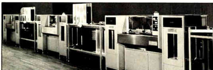
Pass-Thru™ Automatic Board Handling System eliminates manual board feeding and removal. System accepts boards in stack or magazine input, moves them through the machine and accumulates inserted boards in a magazine loader for automatic movement to the next machine.
