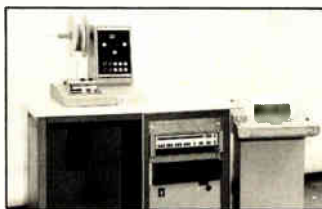
Model 2863 Off-Line Tester. Can be used for inspection of incoming components or sequenced components at up to 36,000 an hour.
