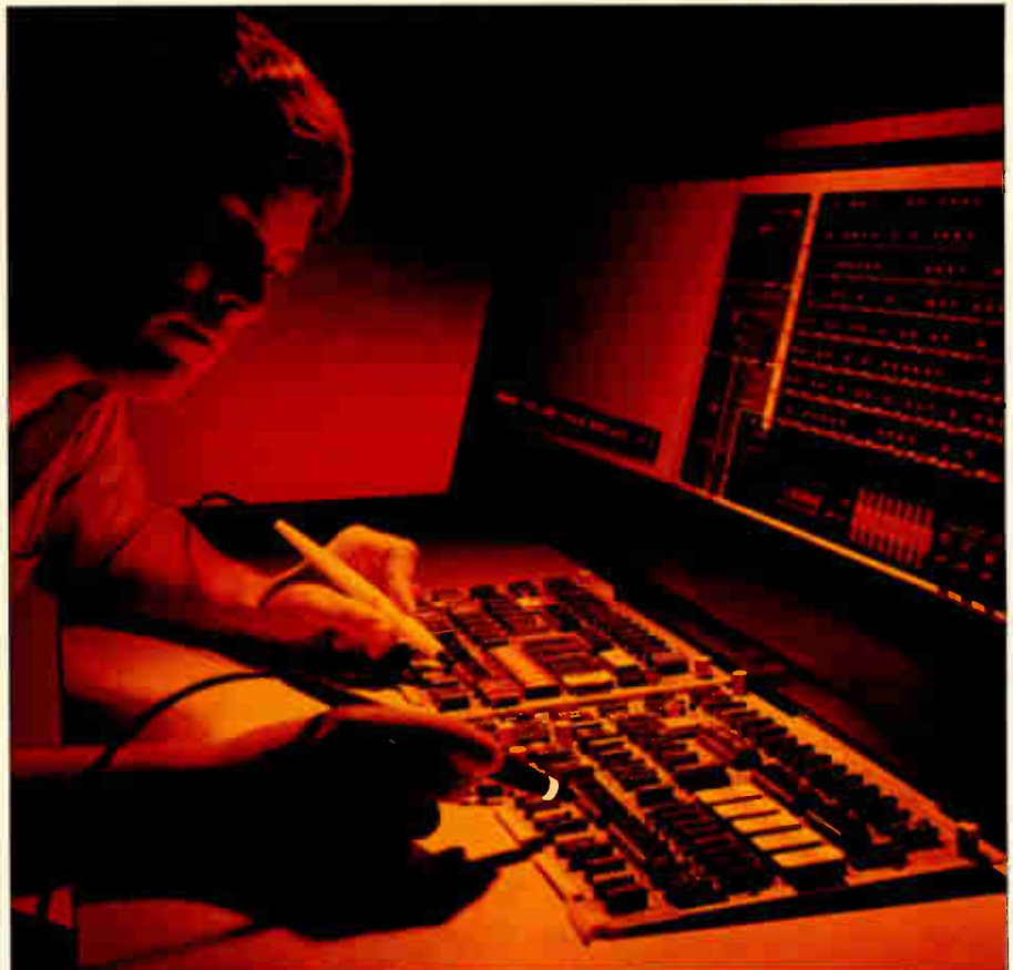
More capable test systems like Fluke's 3050A digital/analog tester can check out a variety of circuitry and permit full test-program generation.
