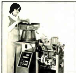
Model 2425/2315 Axial Lead Straightener-Taping Machine. Automatically straightens leads of axial components and tapes them at a rate of 15,000/hr.
