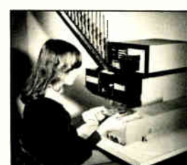
Model 6731 Mod-U-Sert™ Manual DIP Insertion Machine. Easily-programmed built-in memory automatically feeds .300", .400" or .600" DIPs from 12- or 16-magazine feed rack.
