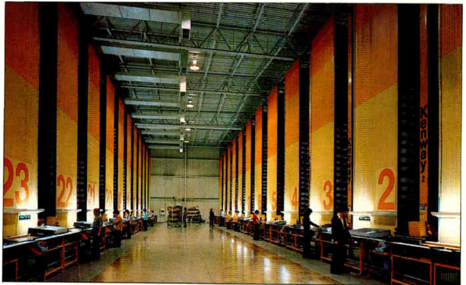
Automated parts-supply systems, such as this one from Eaton-Kenway, can improve material-handling productivity by as much as 50%.
