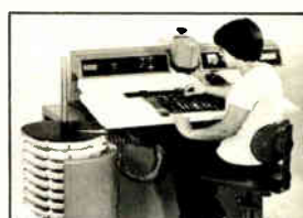
Model 6232 Man-U-Sert Manual Assembly Machine. Machine automatically positions board, shows operator exact location for each insertion, cuts and clinches leads after insertion.
