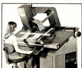
Model 3986/3991 Wire Termination Machines. Panels are positioned under termination gun and indicate wire to operator, for termination rates of 600 to 1200 wires/hr.
