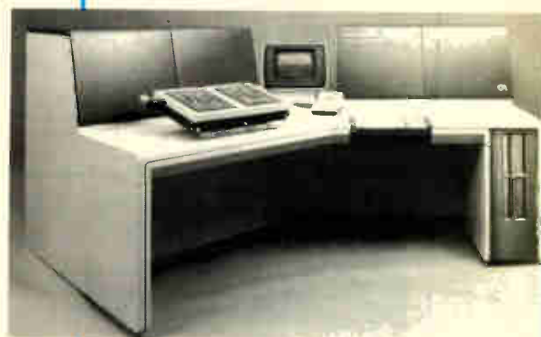
Test sharing. The Marathon network (left) relies on an LSI-4/95 to manage distributed computers in a multitasking mode. A test station may be a prefunctional tester (above) or a functional unit.
