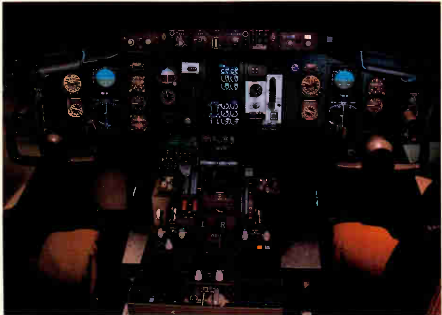
Advanced electronics paves the way for two-member flight crews in the Boeing 757/67, vs. three crew members in earlier commercial craft.
