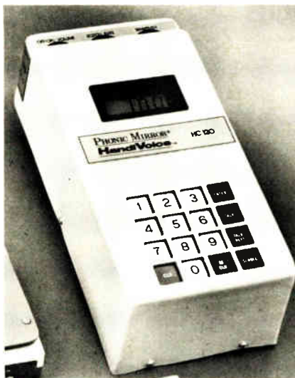
Voices. Calculator-like 4-lb HandiVoice from Votrax, at left, stores and produces up to 40 words keyed in via three-digit codes. For more severely handicapped, larger lap-sized synthesizer, at right, relies on 128 touch-sensitive keypads that correspond directly to specific words. The unit accommodates four different vocabulary overlays.
