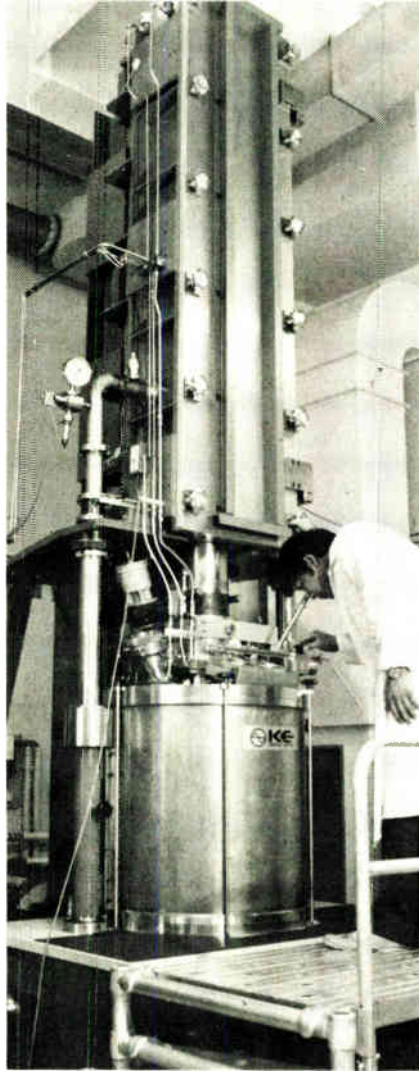
Big melter. Standing 4.5 m high, furnace is turning out 5-in.-diameter silicon ingots
