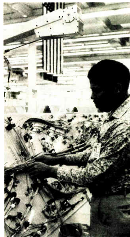
Spotter. Beam projected by overhead laser traces out paths in which wires are laid.
