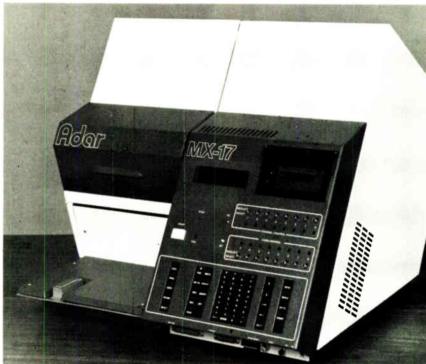
Testy. Small but powerful, new breed of LSI testers like the MX-17 from Adar fit on a tabletop. The testers derive their low cost from the use of LSI in their design. They are also relatively easily programmed in the language being used with the device under test.
