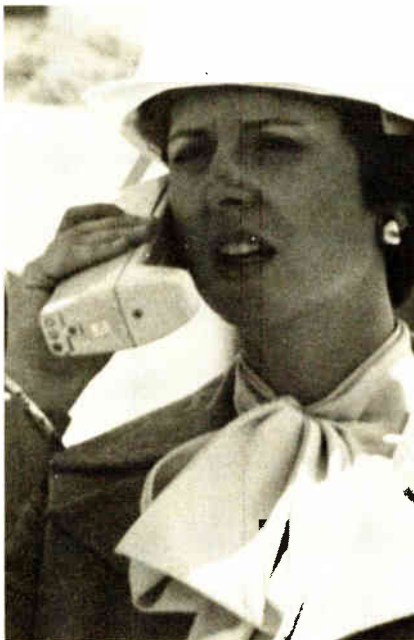
On the air. Motorola's portable radio-telephone is shaped like the traditional home phone handset. It weighs 2 pounds and can fit into a briefcase or purse.
