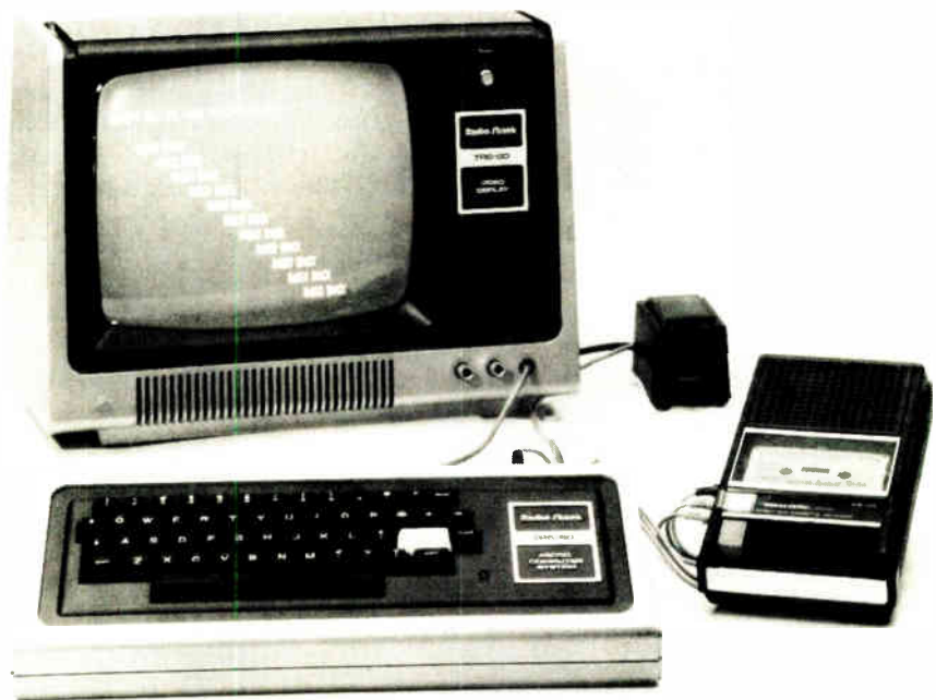
System. Radio Shack's $600 TRS-80 microcomputer system consists of a 53-key keyboard containing a Zilog Z-80 microcomputer, 12-in. video display, data cassette recorder, and regulated power supply. The keyboard unit also sells separately for $400.
