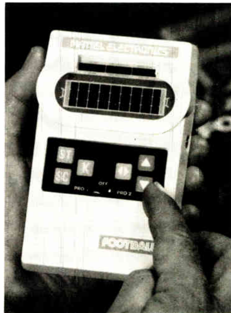
Grid game. In Mattel's football game, moves are made on matrix of LEDs. After each play, scoreboard is automatically updated.
