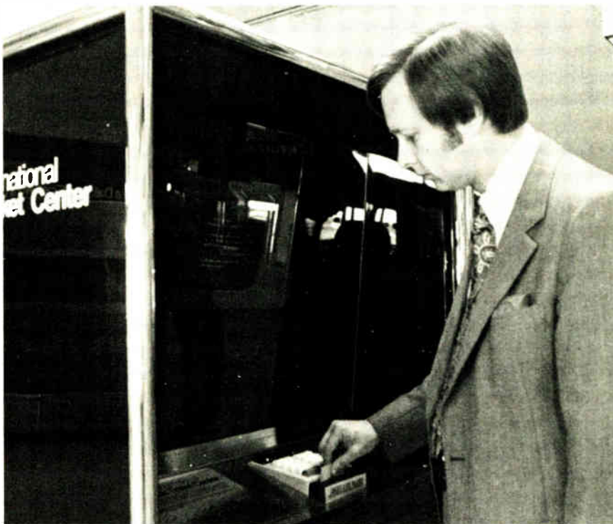
Ticketing agent. Braniff International's Branimatic ticket-issuing machine presents instructions on cathode-ray-tube display and uses slide-through credit-card reader.
