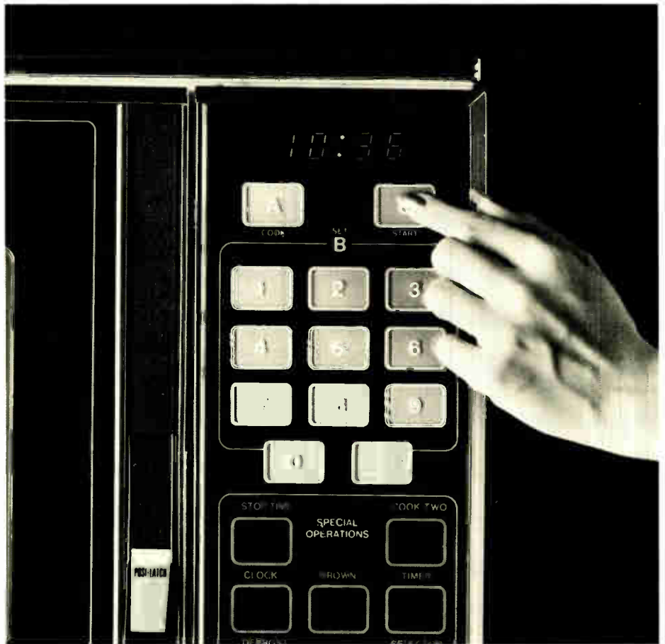
1. Processor cookout. Success of microwave ovens with LSI controls and capacitive glass touchpanels has spurred interest in applications in other appliances. Among the programmable ranges using standard microprocessors are Litton's Model 460 Memorymatic, top, with its control the TMS 1000 from Texas Instruments, and Tappan's Tap 'N Touch, bottom, which uses the TMS 1100 from Texas Instruments.
