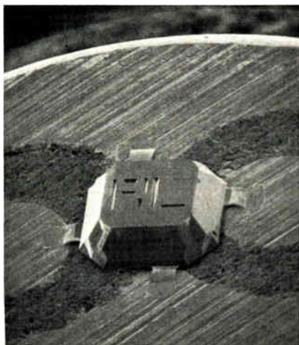
Actual scanning electron microscope picture of a SURE transistor mounted on the newly developed TO-18 header.
