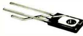
TO-5 PCB Pin Circles (Heatsink Optional) Collector Bent Away From Heatsink Surface
