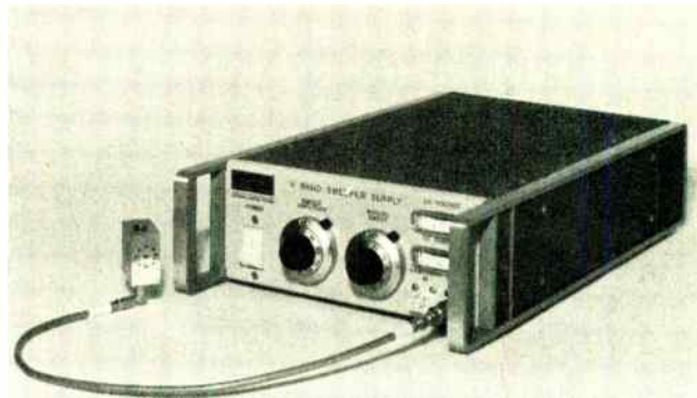
8. And back at the lab. Millimeter-wave sweep generator has Impatt oscillators for laboratory testing. Bias-current tuned, the head is fixed by flexible cable to the power supply.
