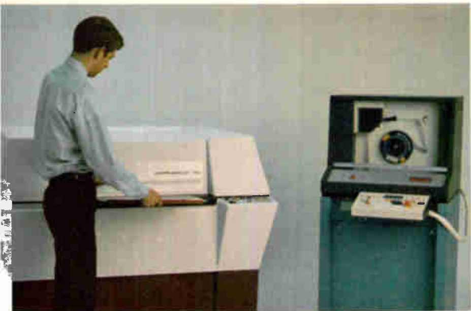
Lights on. Film is housed in a light-tight cassette so the room doesn't have to be darkened during loading and unloading of the machine.
