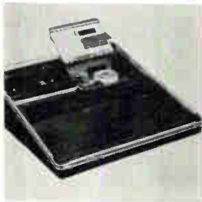
Portable strip printer 5064 is a digital impact unit that can fit into data communications systems to provide hard-copy read-out. It features compactness, printing speed, reliability and economy. Operation is based on the flying hammer principle. A type wheel having 64 characters and associated timing markers rotates continuously. Dataline Inc., King of Prussia, Pa. [402]
