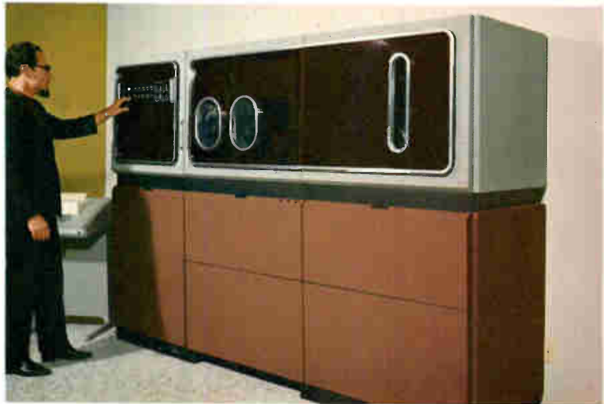
Working up. Small masters, under 6 x 6 inches, are plotted on a 1:1 scale, and others can be enlarged four times up to a size of 22 x 22 inches.
