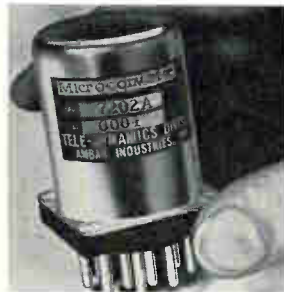
Microconverter 7202A accepts computer levels and converts them to drive commercial communications equipment. The compact unit isolates input power and ground returns from the output by optically coupling input signals through a light-emitting diode and light-sensitive resistor. Price is under $100 in small lots. Tele-Dynamics, Virginia Dr., Ft. Washington, Pa. [403]
