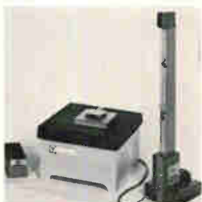
Nondestructive testing system, which can measure flatness differences as small as one ten-millionths of an inch, speeds photo-mask production. Test is made without touching the active surface which may be opaque, transparent, conducting or nonconducting. Calibration is traceable to the National Bureau of Standards. Towne Laboratories, U.S. Hwy 206, Somerville, N.J. [422]
