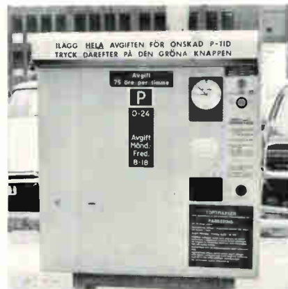
Vendor. Coins inserted in slot at upper right of Parkomat trigger logic circuits, on removable cards in long box at top, and ticket printer (center).
