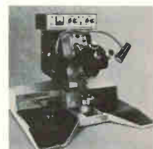
Improved version of the model 484 wedge bonder can bond 4,000 semiconductor wires per hour. It offers solid state control circuitry and photocells to take the place of carbon brushes. Descent rate of the tool at the moment of bonding has been slowed for better control and to prevent excessive wire deformation. Kulicke & Soffa Industries Inc., Fort Washington, Pa. 19034 [428]
