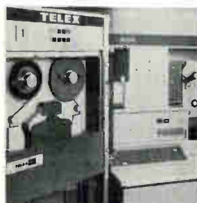
Multiformat read-only tape drives 4853 and 4863 are available with 1600 characters per inch capability for computer output microfilm systems. The 4853 offers a 75 inch per second tape speed and a maximum transfer rate of 120 kilobytes. The 4863 is faster at 112.5 inch per sec with a maximum transfer rate of 180 kilobytes. Telex Computer Products Division, Tulsa, Okla. [407]
