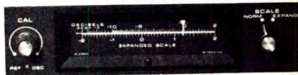
Switch-selected meter modes, normal or expanded scale, provide level measurement resolution of 0.05 dB. Signal generator level increments as fine as 0.01 dB can be readily resolved.
