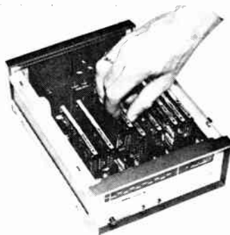
Modular. Multiplexer board is added to expand capability of converter.
