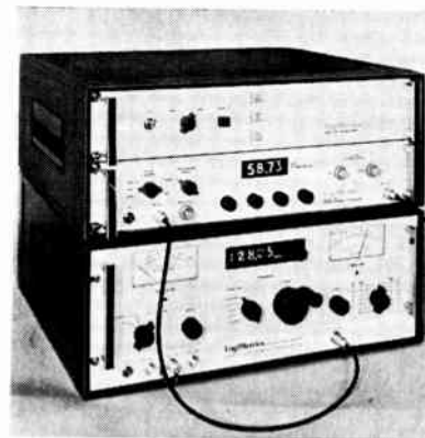
Automatic. System for frequency measurement includes generator, at bottom, plus attenuator and programmer.
