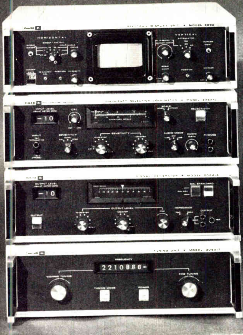
Three 4-kHz channels of L3 carrier multiplex system. Center channel has teletype subcarriers. Model 360A is in 12-kHz sweep width mode, sweeping from 6.780 to 6.792 MHz.
