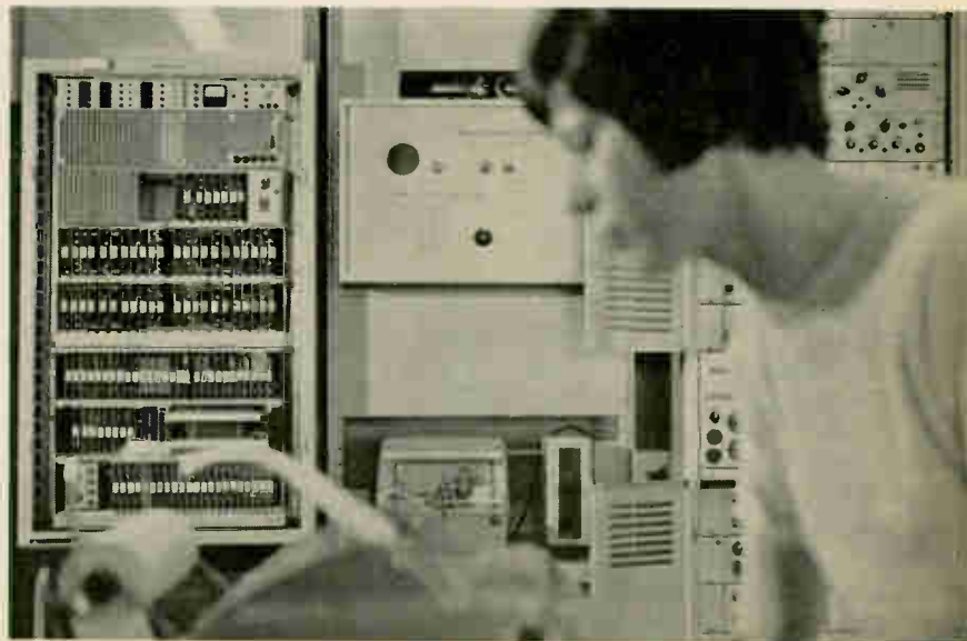
Siemens' teleprinter buffer with magnetic-core matrix replaces as many as four conventional paper-tape reperforator units.
