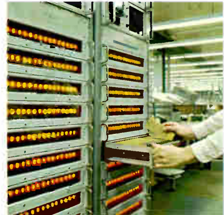
Decade counting assemblies for all solid-state counters undergo a temperature of 80°C for 2 hours to force failure of any marginal components. Despite this torture, the failure rate of decades is less than 0.5%. The assemblies are also operated for 22 hours at room temperature.
