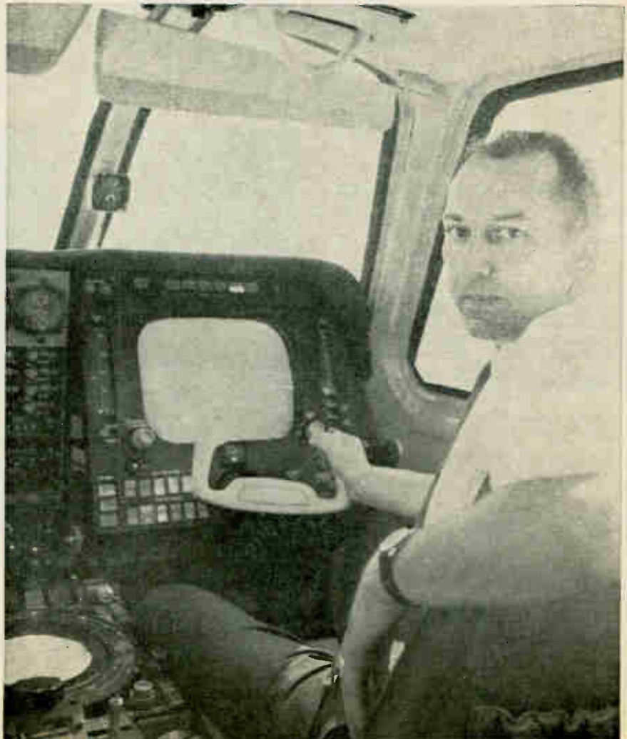
Contact analog display in a Twin-Bonanza J-50 after a test flight by Willis Dworzak, engineer for the Advanced Aircraft Instrumentation System program. The vertical panel and horizontal situation display at pilot's left gives him almost all the information he needs to fly the plan
