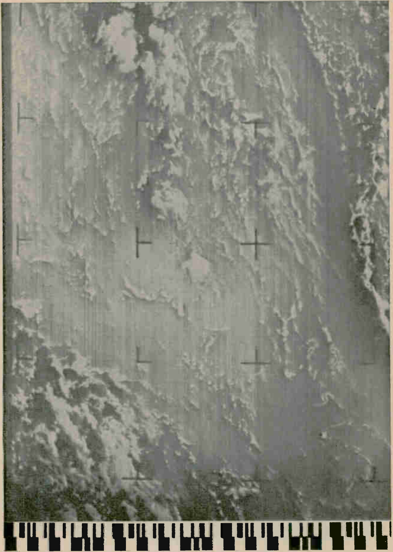
Cloud cover photograph taken by Nimbus 2 cameras. The coded signal (bars and spaces) provides time and orbital information to ground stations. The station operator uses this data to determine the spacecraft's location.
