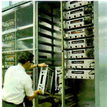
To force any marginal components to fail before shipment, all solid-state counters are operated at +65°C for at least 16 hours in heated cabinets.
