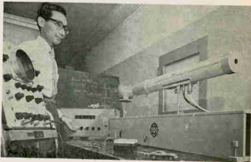
Hitachi laser unit translates contours into digital dimensions. Tube housing laser and detection system moves in and out to keep beam focused on surface.
