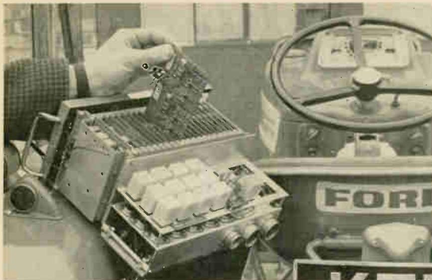
Tractor-mounted receiver picks up binary-coded control signals.
