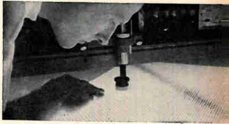
Master pattern is cut from artwork film by drafting machine. The pattern, being inspected by a technician, is paired with a similar pattern and modified to create wiring layouts for multilayer circuit boards.
