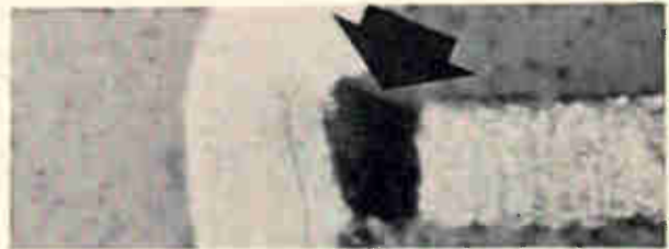
Vertical section through one side of a hole exhibits a discontinuity caused by improper cleaning; a blob of epoxy isolates the hole plating from the pad.
