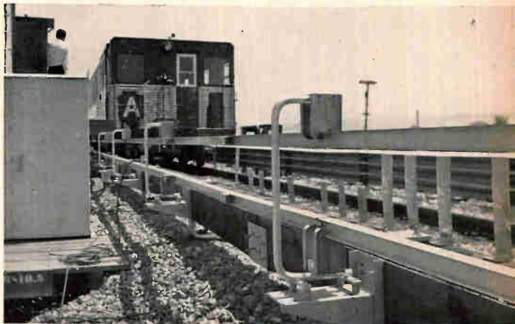
Philco's automatic control system determines the train's location by recognizing combinations of tall and short pickets it passes.
