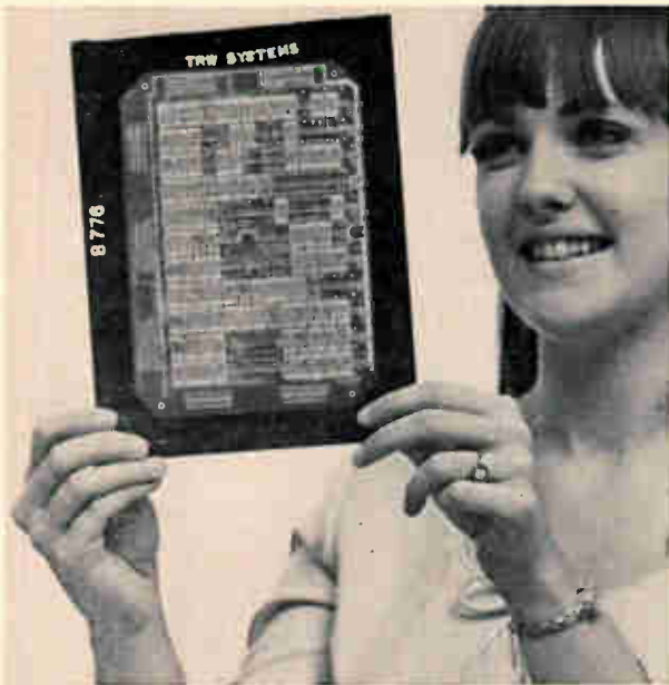
Perfect appearance (of the multilayer board, of course) is what an inspector looks for in X-ray film.
