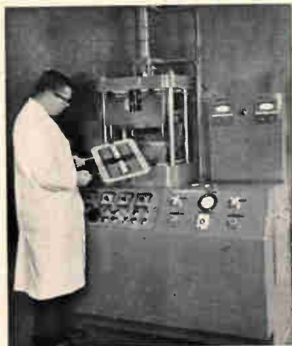
This 25-ton 359D packaged system includes molds, loading frames, and controls for economical, direct encapsulation by transfer molding.
