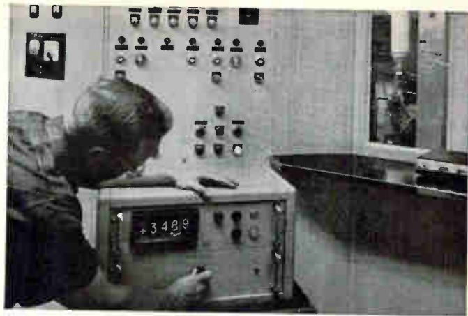
A "start-up" system, composed of an NLS V60 Digital Millivoltmeter and selector switch with built-in normalizers, is used to adjust each engine's operating conditions to standard values prior to connecting that engine into the automatic system. Above, a pressure of 34.89 psi is being displayed.
