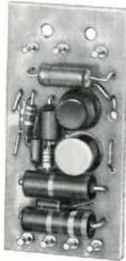
"DC Pulse Circuit" produces square wave millisecond pulse for high speed devices. Data Sheet 194.
