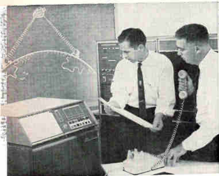
COMPUTER ENGINEERS send messages from an IBM 1401 in Endicott, N.Y., to a 1401 in France by Telstar. Other channels were used for voice communications
