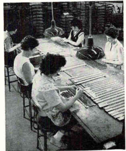
LEAD INGOTS are used to hold components during manufacture
