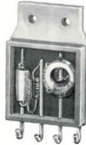
"One-Shot" produces one square wave of 0.1 to 10.0 microseconds regardless of actuation speed. Data Sheet 150.
