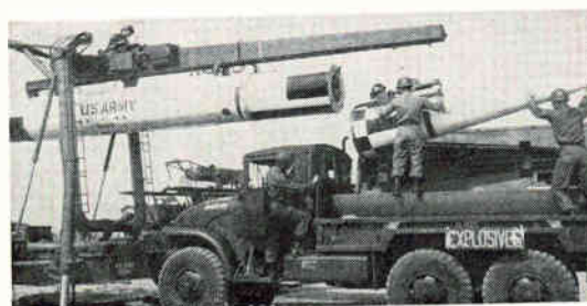
WARHEAD SECTION being removed from container and mated to rest of Sergeant missile on mobile erector-launcher
