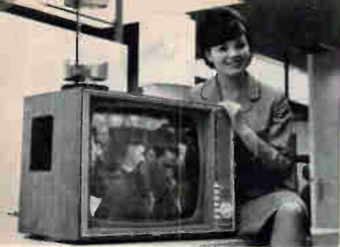
Uhf antenna consists of two bow-tie dipoles; plastic hood makes antenna into lamp (Telefunken)
