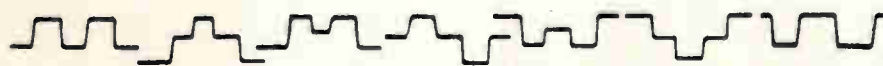
A few of the mixed output possibilities: 0.5 \mu s wide; 25 v pulses; 93 ohm load.
