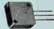
½" Square Resiston Carbon Trimpot—Model 3251. Operates to 150°C / L, P, W terminals / ½ watt / 20K to 1 Meg. Sealed. Meets Mil Specs for cycling humidity.
