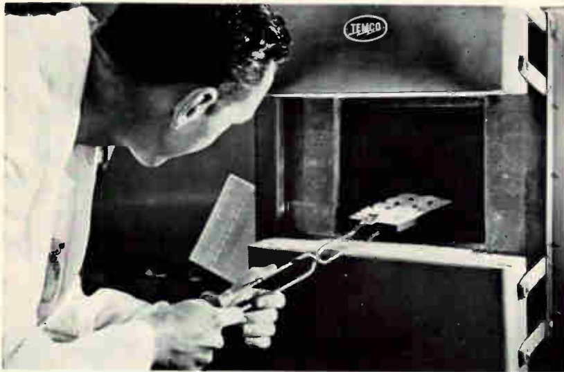
Molten-salt process is used at Lockheed to metalize titanium film on inorganic substrate. Electroplating another metal on substrate develops terminations and photoetching converts selected areas to resistive or dielectric materials to form all passive electronic components
