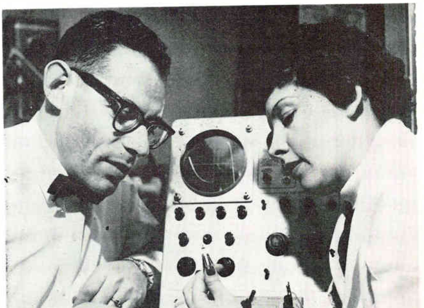
Physicist and a technician examine a new gallium arsenide tunnel diode under test. Characteristic E-I curve is seen on oscilloscope
