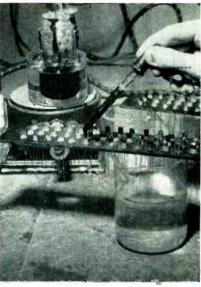
Potting germanium diodes with mixture of resin and lampblack, kept at 120 C with an oil bath on hot plate in background. Beaker in foreground merely serves as support for plastic strip holding diodes
