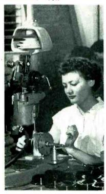
Foot-controlled air cylinder, replacing feed handle of drill press, leaves both hands of operator free for holding and indexing meter cases being drilled
