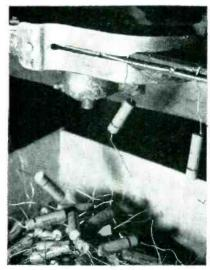
Claw-type device for removing dipped capacitors from coil spring as the spring moves from right to left through the
