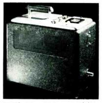
Portable vapor detector powered from wet battery was developed for atomic energy program
