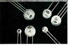
Ceramic Disc Hi-Kap Capacitors hold thickness to a minimum . . . have very high capacity in extremely small size. Use in h.f. circuits for bypass and coupling. Ceramic body assures low inductance. Other characteristics—humidity resistance, power factor, etc.—similar to BC Tubulars, Bulletin No. 42-4R,
