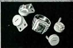
Centralab Ceramic Trimmers meet applicable portions of JAN-C-81. Very small size. Screw driver adjustment over full capacity range (180° rotation). Maintain stability in any position and under vibration. Spring pressure contact for rotor and stator. Bulletin No. 42-101.
