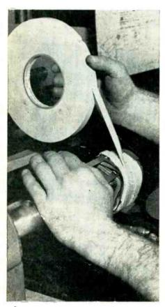
ANCHORING sheet leads on this PECO transformer coil requires a strong but not bulky tape. The job is done to order with "Scotch" Electrical Tape No. 45. Sheet leads can be punched, then wired directly to the transformer. No terminal bond is needed.
