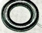
O.D. 1-5/8" x 7/8" I.D. Wire—38 AWG Winding Speed—800 rpm
