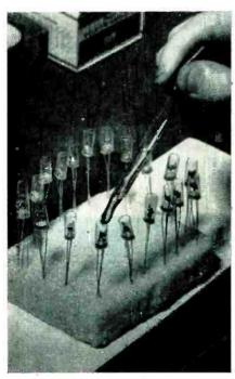
Using medicine dropper to fill each transistor sleeve with potting resin
