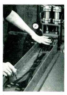
Setup using two air cylinders and longer trough for checking submerged cables for air leaks
