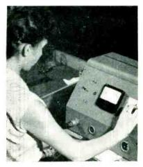
Method of using insulation resistance test set with adapter (in box underneath) for checking five cables at a time
