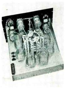
Transmitter final amplifier uses single 4-250A tetrode
