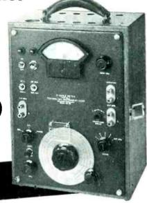
The type 310A Z-Angle Meter measures impedance directly in polar coordinates as an impedance magnitude in ohms and phase angle in degrees: Z  $\underline{/\theta}$ Impedance Range: .5 to 100,000 ohms, covered by a single dial and a four position range switch.
