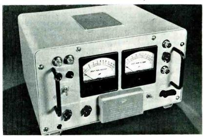
Nonlinearity of velocity scale makes two meters necessary to cover range from 3.5 to 35 ft per sec
