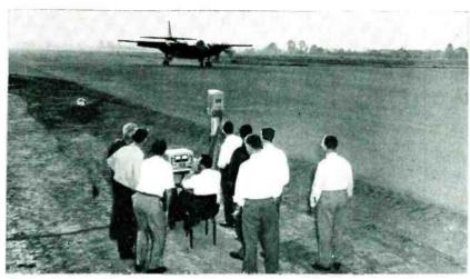
Two-unit descent indicator measures time required for plane to descend one foot
