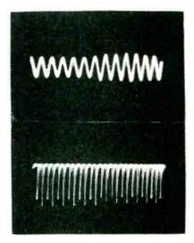
Sine-wave input at top, results in series of sharp negative peaks in the output
