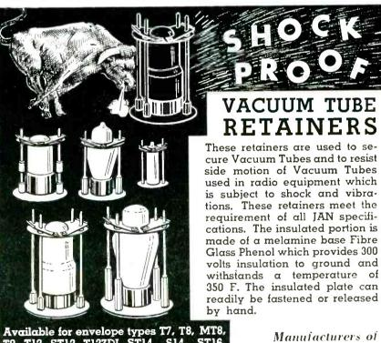
Available for envelope types T7, T8, MT8, T9, T12, ST12, T12ZDI, ST14, S14, ST16, T51/2, T61/2, MT-IC, ST19, T14, ST128CT-9.
