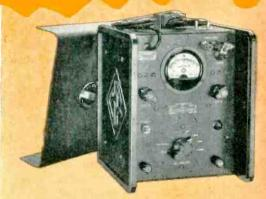
Ir sulation Resistance is measured directly by the Type 1362-A Megoh neter at the commonly accepted ASTN potential of 500 velts.
