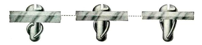
Spring-Lock—the easy-to-use removable fastener for modern designs—works whether panel thicknesses run over or under specifications! Spring wire deflects automatically to handle greater or lesser thicknesses. Spring-Lock's design flexibility makes it more than a fastener: it can be adapted as a shelf support, door strike, knob or any similar panel-mounted device. Many standard shapes and sizes of Simmons Spring-Locks are available from stock.
