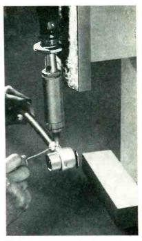
Vertical support for soldering iron used in soldering ferrules of cable shield to shell of connector plug
