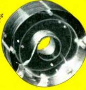
Stycast 1030 CM A tough, black, rubbery material with high impact strength for embedments used over a temperature range from -90°C. to +170°C. Monopole transformer at left sealed in Stycast 1030 CM.
