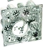
A five tube superheterodyne in volume production utilizing multiple soldering and semi-automatic assembly techniques . an excellent application of printed wiring methods by Raytheon Manufacturing Company.
