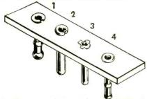
Multi-swage terminals may be assembled by the following methods: 1. flared; 2. rolled; 3. slitted, or 4. spun. Courtesy The Bead Chain Manufacturing Co., Bridgeport, Conn. (336)
