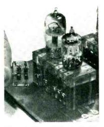
FIG. 1—Cellular technique for mechanized wiring employs three-terminal molded cells that fit into two-tube building block. Printed wiring is used on base plate. Extensions of tube-socket springs make contact and hold blocks in place
